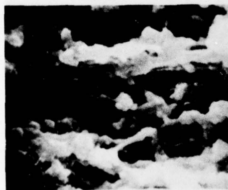
Fig. 6 - SEM photographs of a tear tip in a polybutadiene rubber 24 hrs after cutting. Photograph D is of the tear wall.
