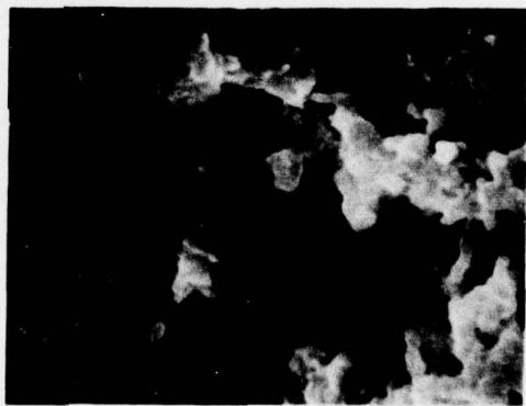
Fig. 4 - SEM photographs of a tear tip in a nitrile rubber 2-3 weeks after cutting
