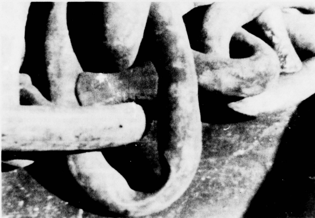
Figure 2. Wear of 3½-inch (9-cm) grade-3 chain used in single-buoy mooring system in North Sea.
