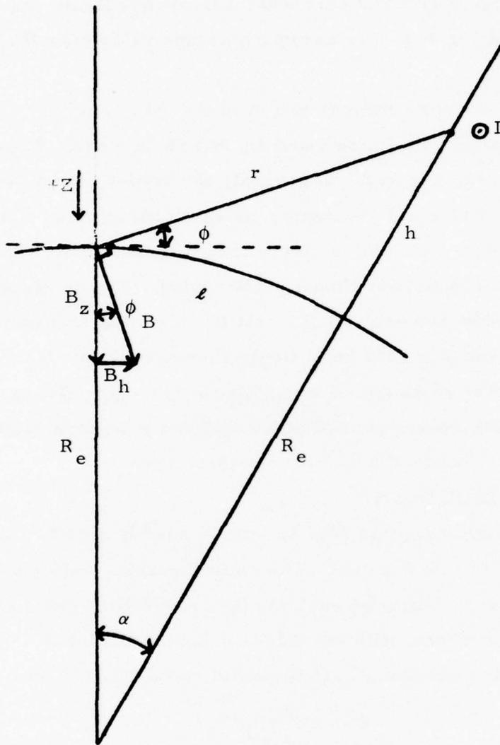
Fig. 3.2 Geometry of the Electrojet Relative to a Single Magnetometer Station in a Cylindrical Earth Model.
