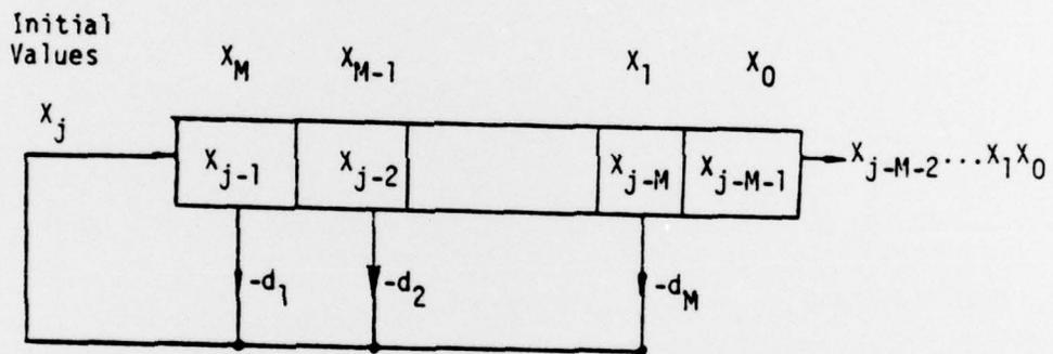
Figure C-2. Linear Feedback Shift Register (LFSR) representing  $\frac{C(z)}{D(z)}$ .
