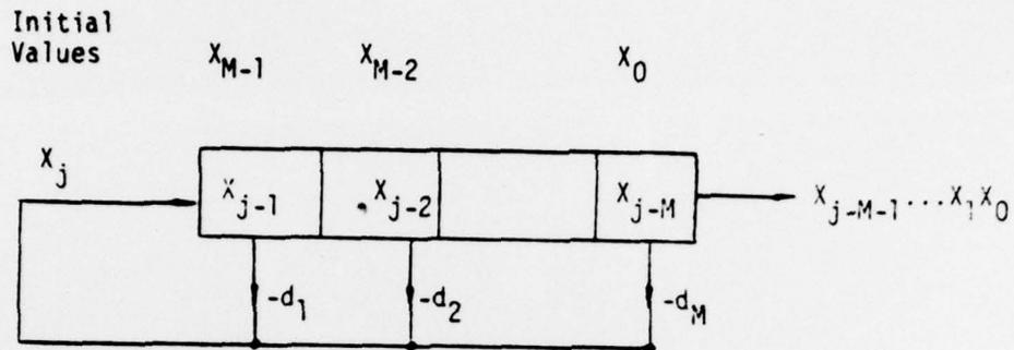
Figure C-1. Linear Feedback Shift Register (LFSR) representing  $\frac{C'(z)}{D(z)}$ .
