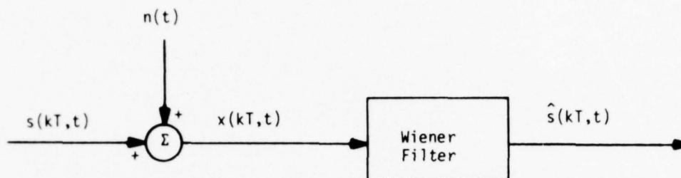
Figure 4-1. Short interval Wiener filtering.
