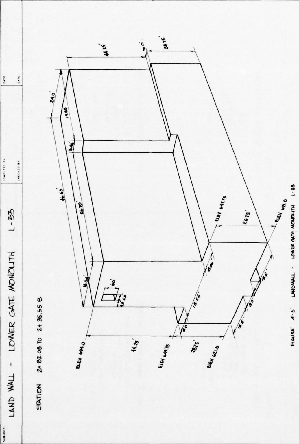
FIGURE A-5 LANDWALL - LOWER GATE MONOLITH L-33
