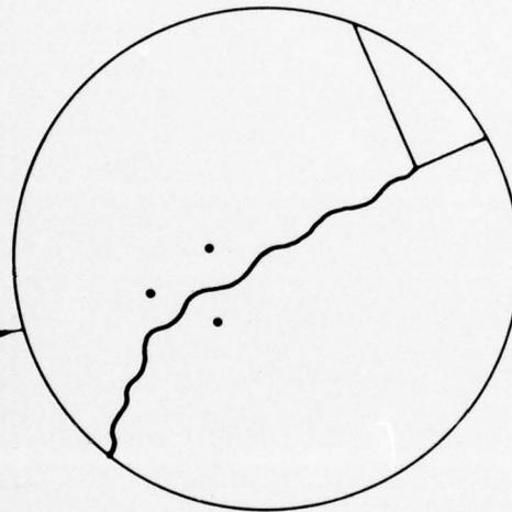
Figure 2.4. Crack and gage locations for strain instrumentation in the river wall gate bay monolith, R-12.
