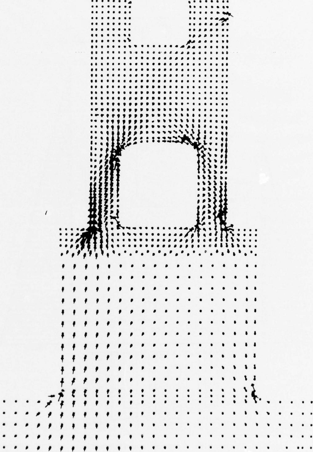
Figure 6.9. Monolith M-8, total stress distribution, normal operating case.
