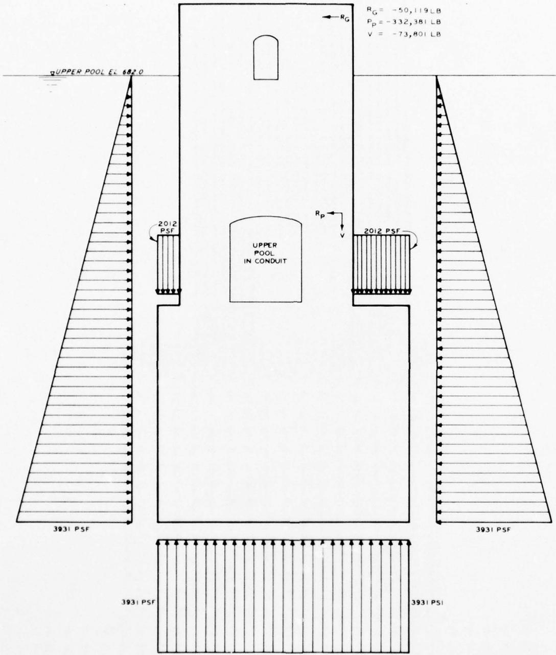
Figure 6.17. Loading, monolith R-12.
