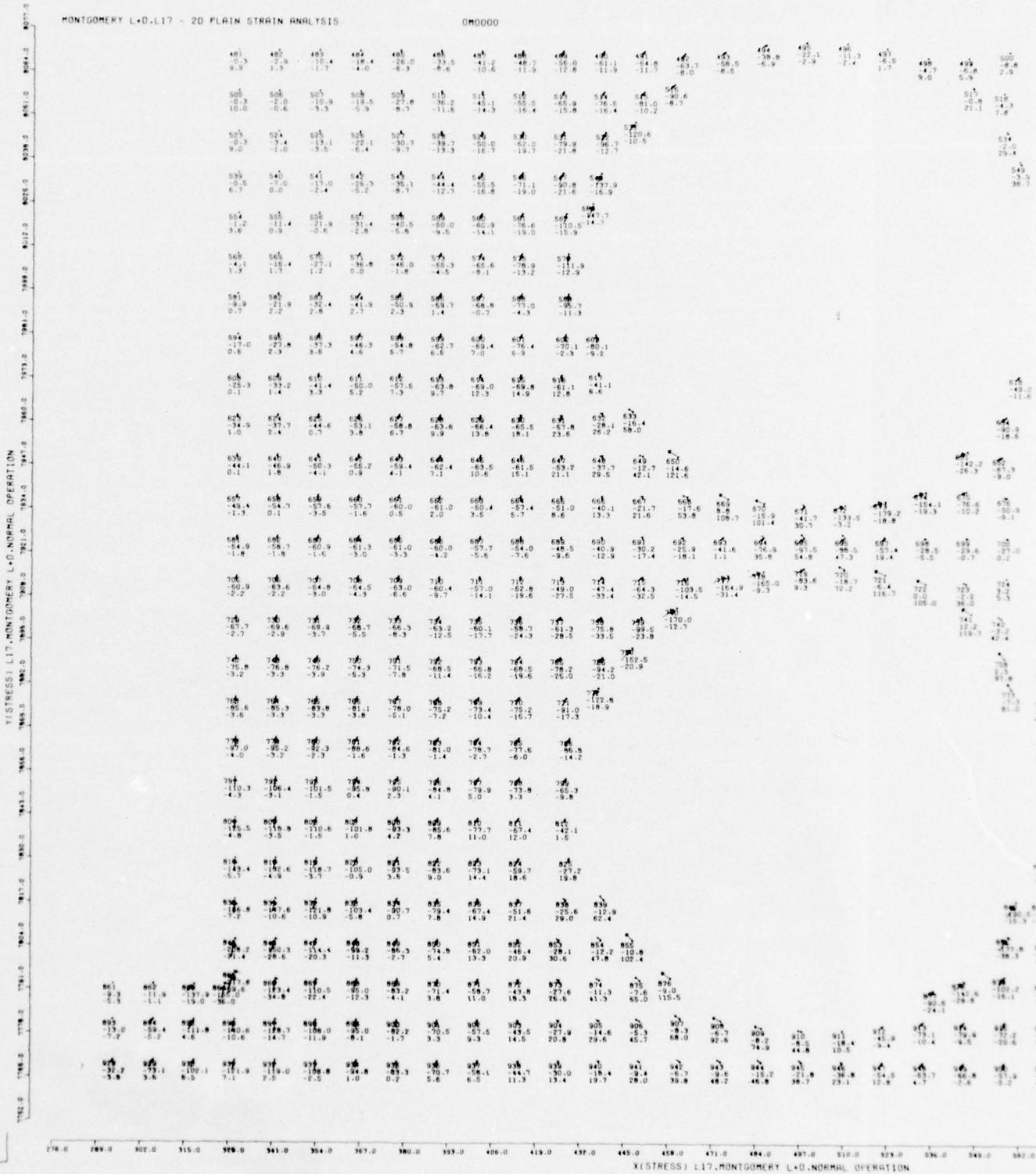
Figure 6.6. Monolith L-17, area of stress concentrations as by area "A" normal operating case.
