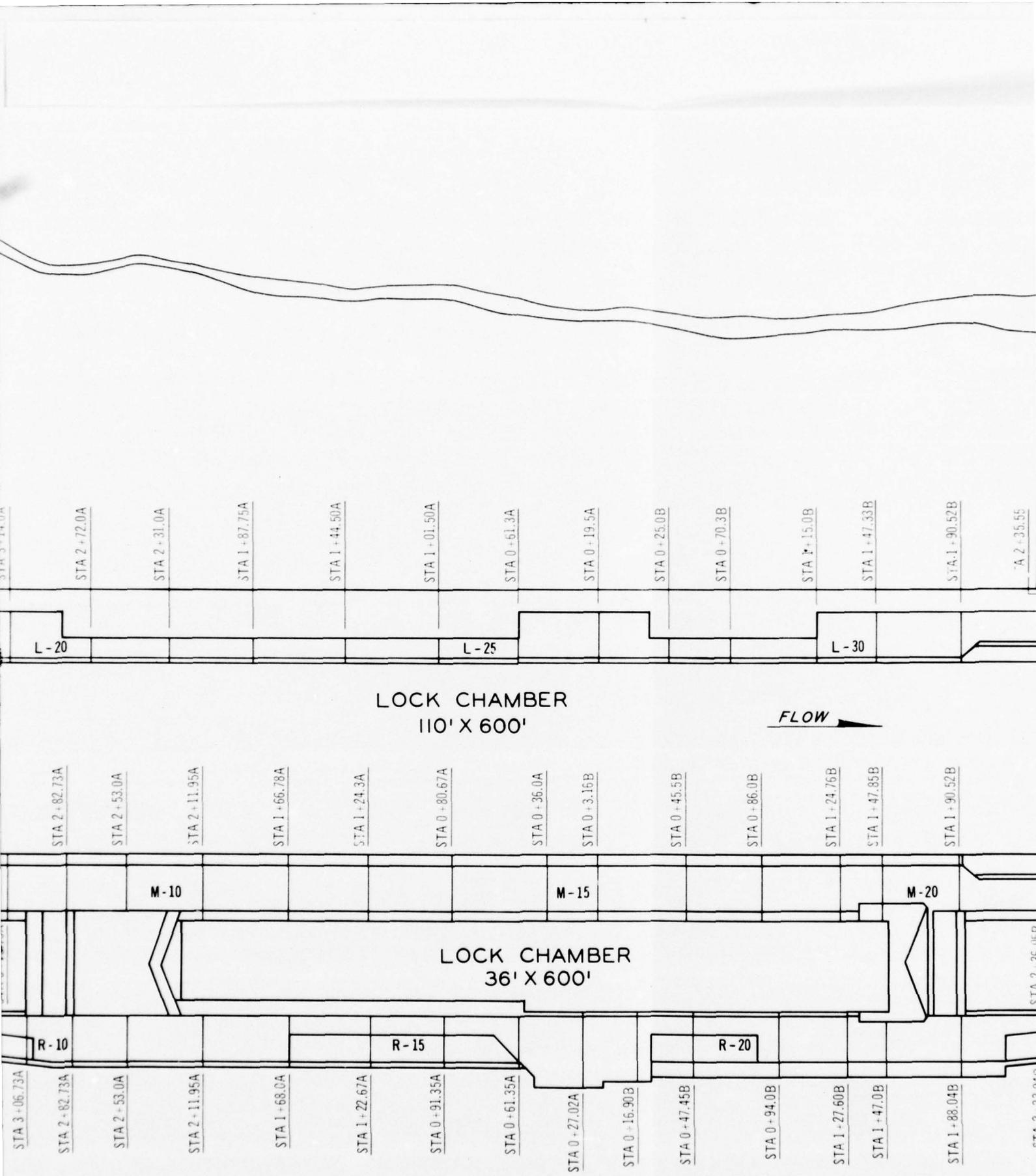
Figure 2.1 Montgomery Lock - monolith and station numbering
