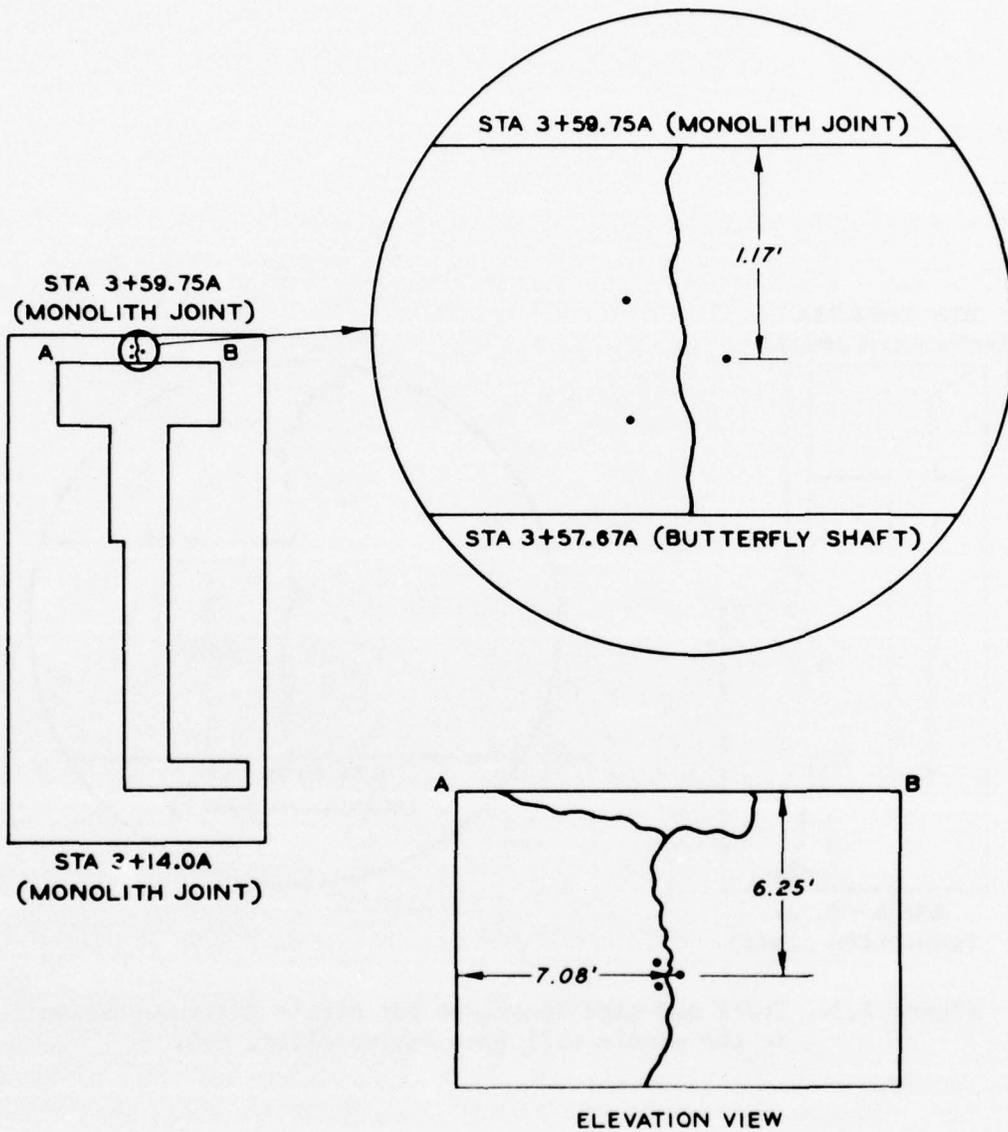
Figure 2.2. Crack and gage locations for strain instrumentation in the land wall butterfly valve monolith, L-19.
