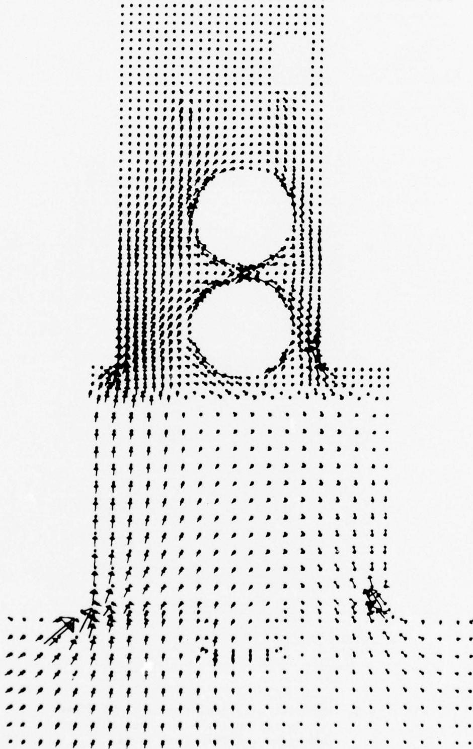
Figure 6.4. Total stress distribution L-17 dewatered.
