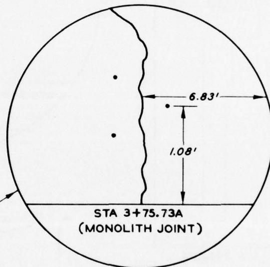
Figure 2.3. Crack and gage locations for strain instrumentation in the middle wall gate bay monolith, M-5.
