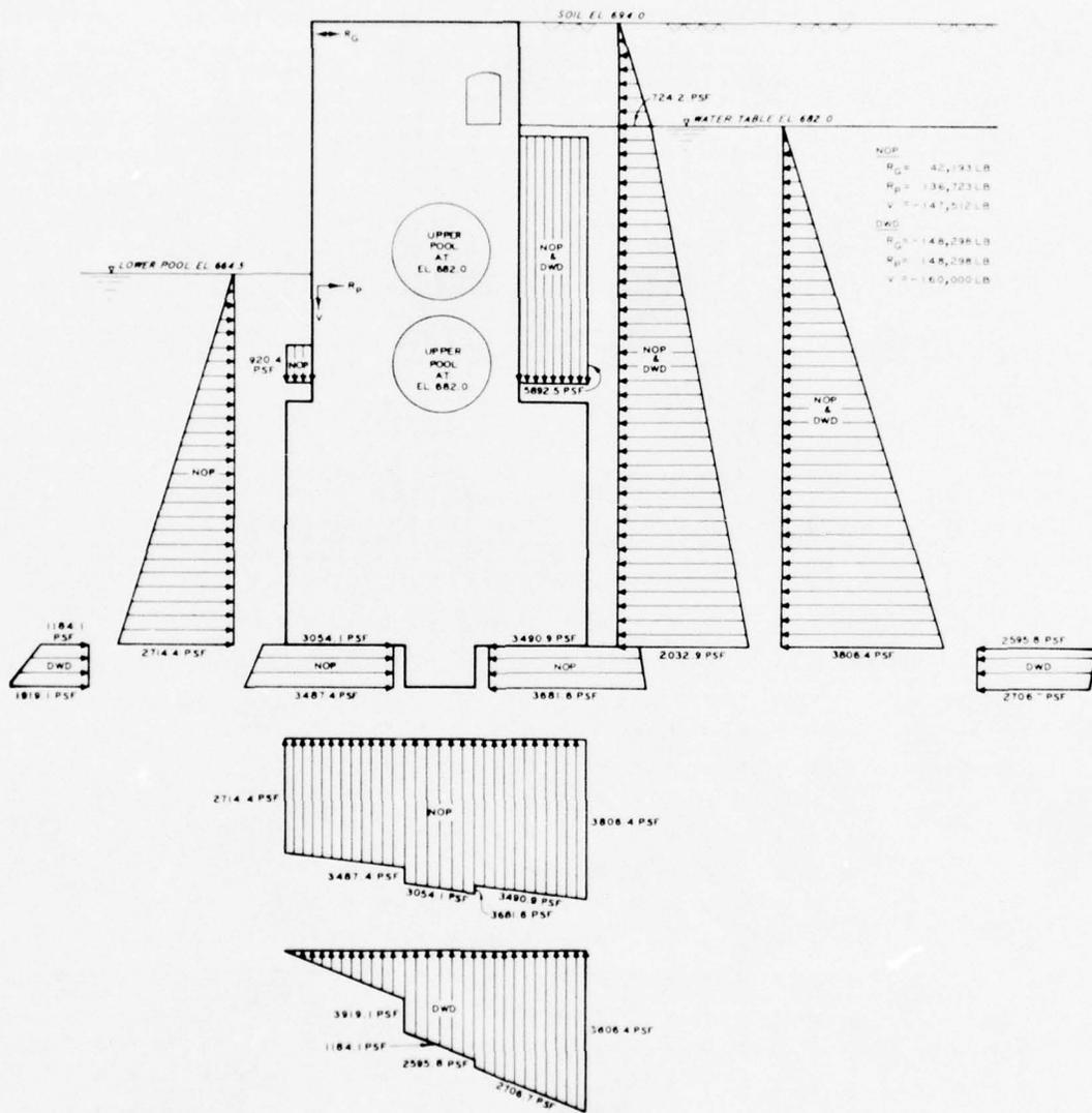
Figure 6.2. Loading, monolith L-17.
