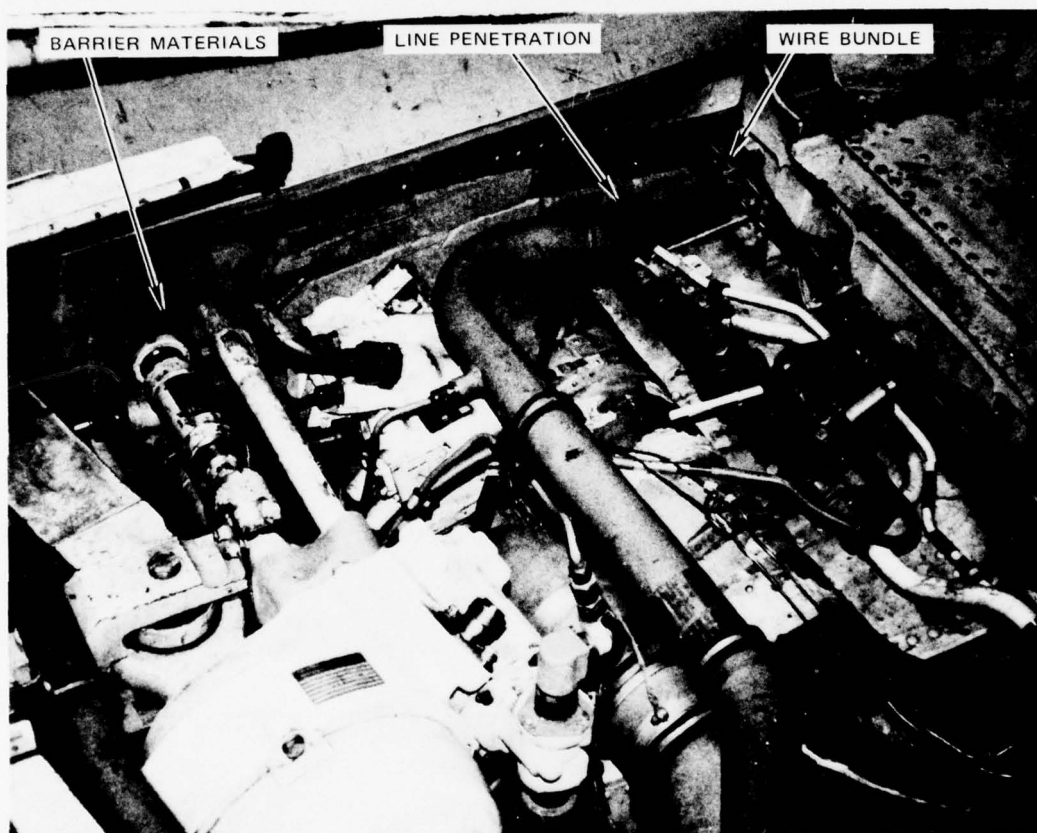
FIGURE 1. Typical Penetrations in a Fire Barrier Installation.
