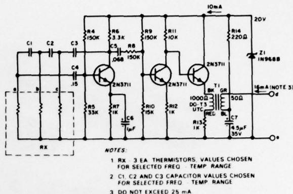
Fig. 7. Schematic of variable frequency thermometer (After Squier 1967).
