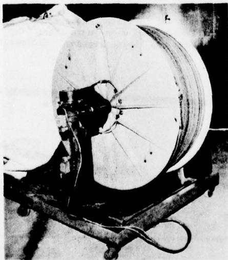
Fig. 6. A profiling winch used in this experiment.
