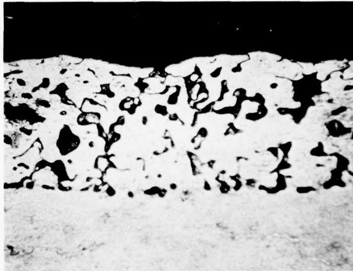
NiCrY coated TDNiCr-1219C/4 hr #13 glass beads, 15 psi - 1 minute.
