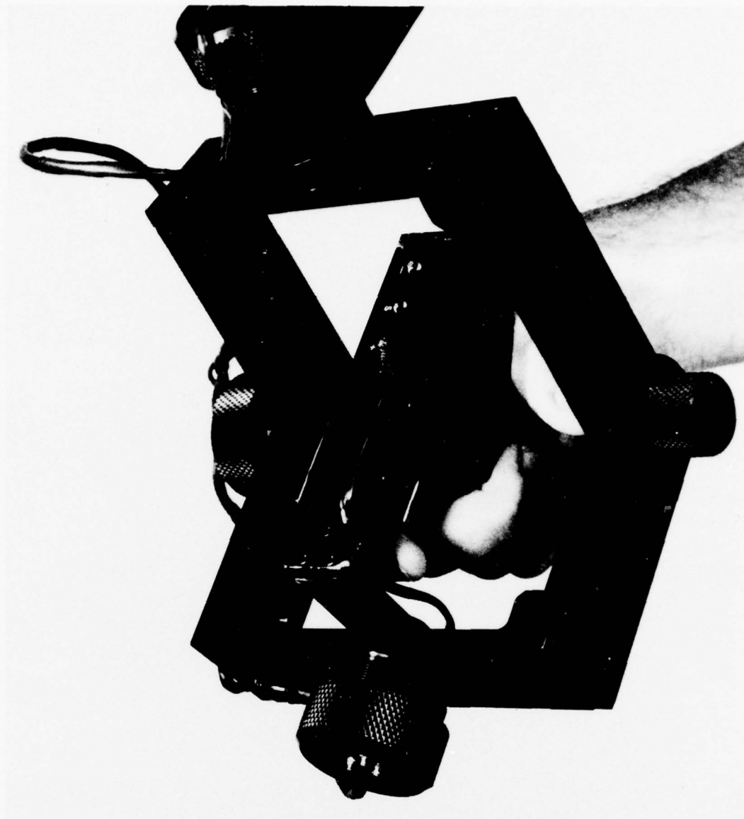
Figure 13. Pistol-grip terminus control for main RUWS manipulator. 2494-4-72
