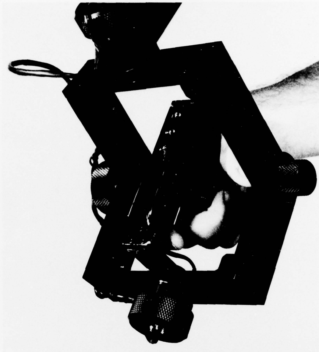
Figure 13. Pistol-grip terminus control for main RU/WS manipulator. 2494-4-72
