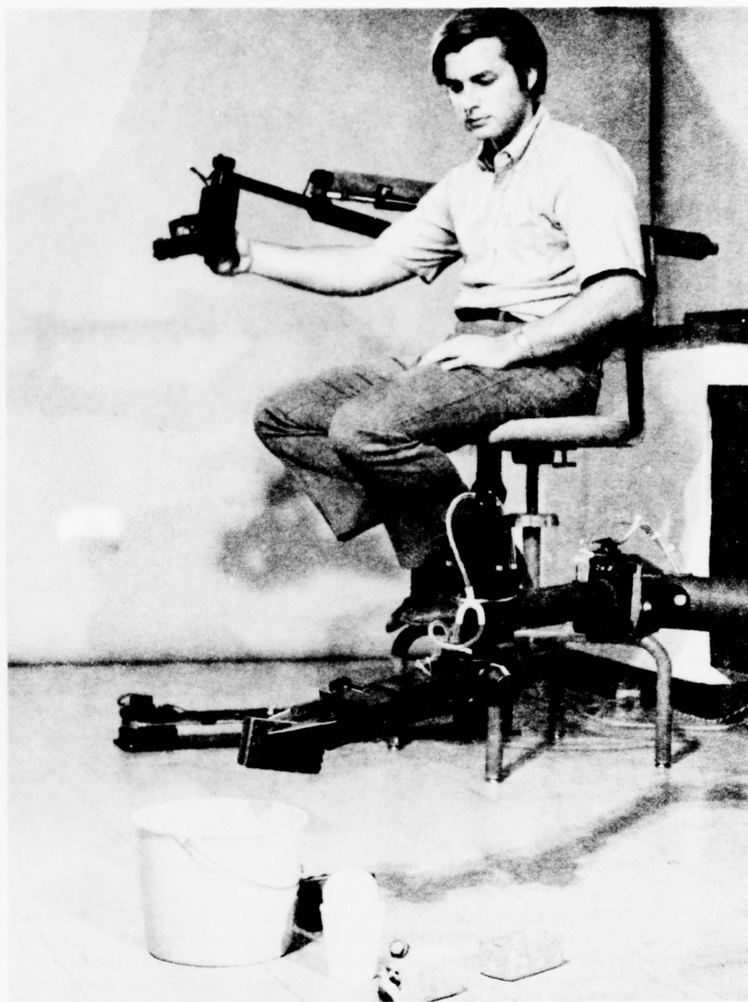
Figure 14. Controller and main RUWS manipulator during laboratory testing. 2588-3-72
