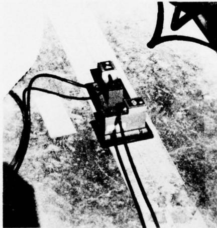
Figure 5. Accelerometers used to measure motion of dam
