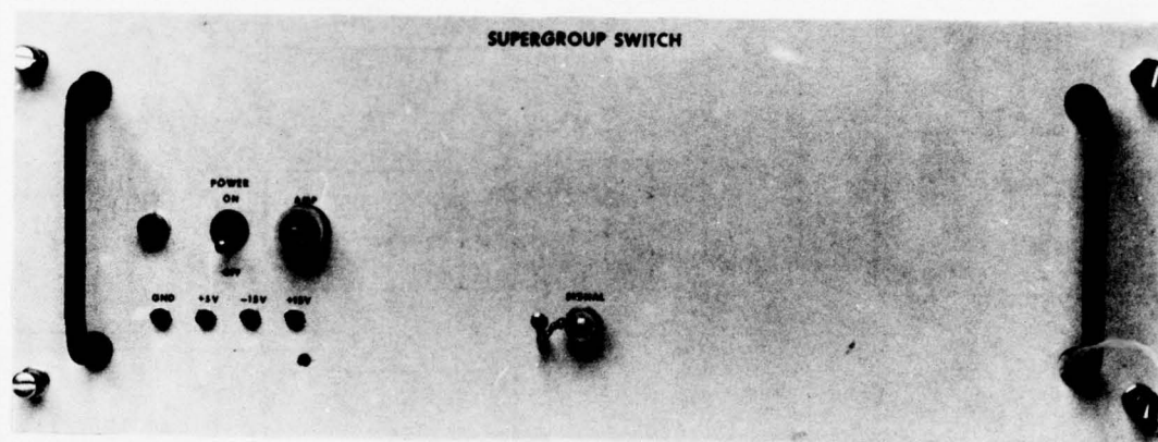
FIGURE 4-41. SUPERGROUP SWITCH, FRONT VIEW
