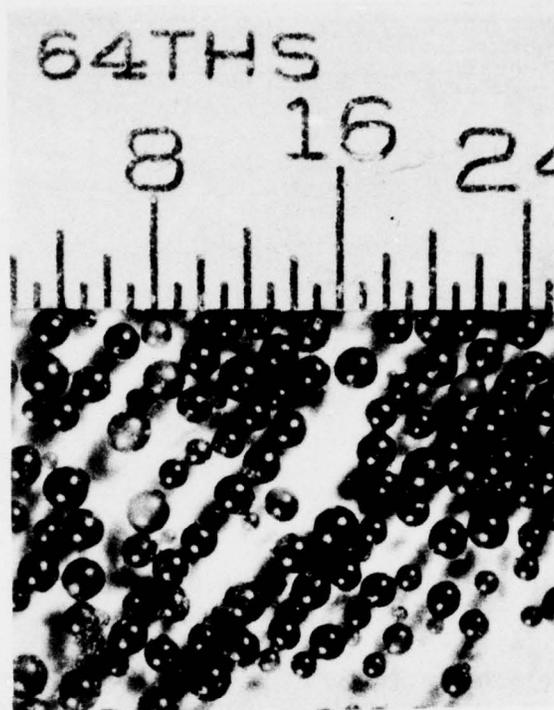
Figure 2. Typical sealing additive sphere size distribution obtained from spray process.
