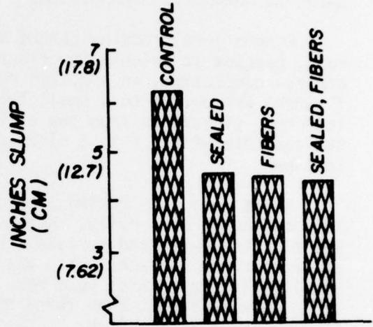
Figure 4. Average slump (in.) for four mix designs.
