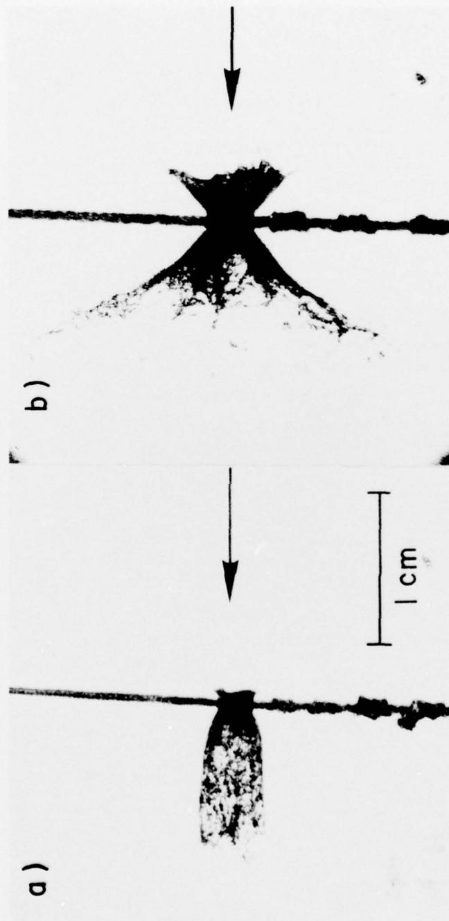
Fig. 6 — Shadowgrams showing the disintegration of polyethylene sheet targets 0.5 mm thick after irradiation with Nd/glass laser pulses. (a) 4  $\mu$ sec after peak laser power, energy  $\sim$  80 J with no prepulse; (b) 4  $\mu$ sec after peak laser power, energy  $\sim$  80 J with prepulse at 600 nsec. Nd/glass laser incident from the right. Exposure time  $\sim$  16 nsec.
