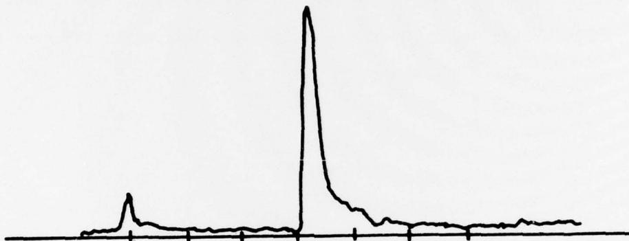
Fig. 1 — The Nd/glass laser pulse produced using Pockels cells to achieve Q-switching. The total pulse energy is  $\sim 100$  J and the width at half maximum power is  $\sim 40$  nsec. The prepulse contains  $\sim 15\%$  of the total energy and occurs  $\sim 600$  nsec before the mainpulse. The beam divergence was  $\sim 0.3 \times 10^{-3}$  rad.
