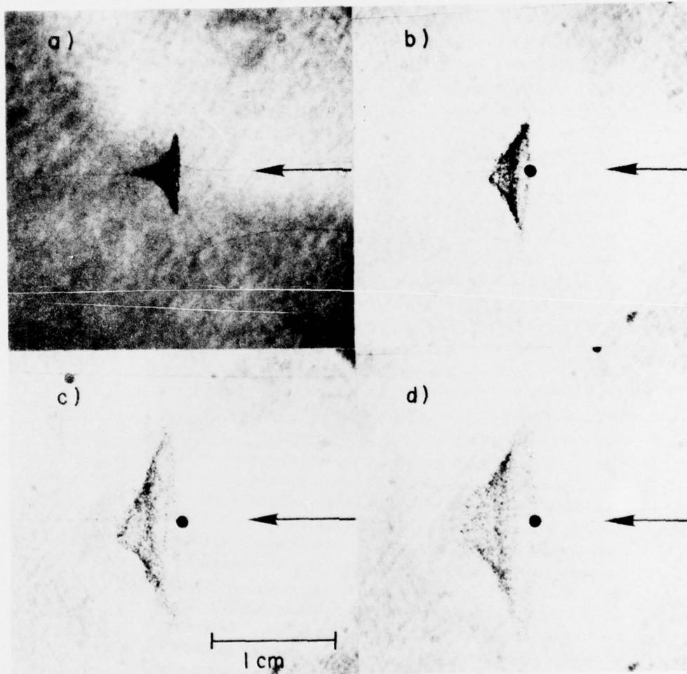
Fig. 2 — Shadowgrams showing the disintegration of 1 mm diameter polystyrene resin beads after irradiation with  $\sim 95$  J Nd/glass laser pulses with no prepulses. (a)  $2 \mu\text{sec}$  after peak laser power; (b)  $4 \mu\text{sec}$ ; (c)  $6 \mu\text{sec}$ ; and (d)  $8 \mu\text{sec}$ . Exposure time  $\sim 16$  nsec. Nd/glass laser incident from the right. The spot in (b), (c), and (d) marks the initial position of the target.
