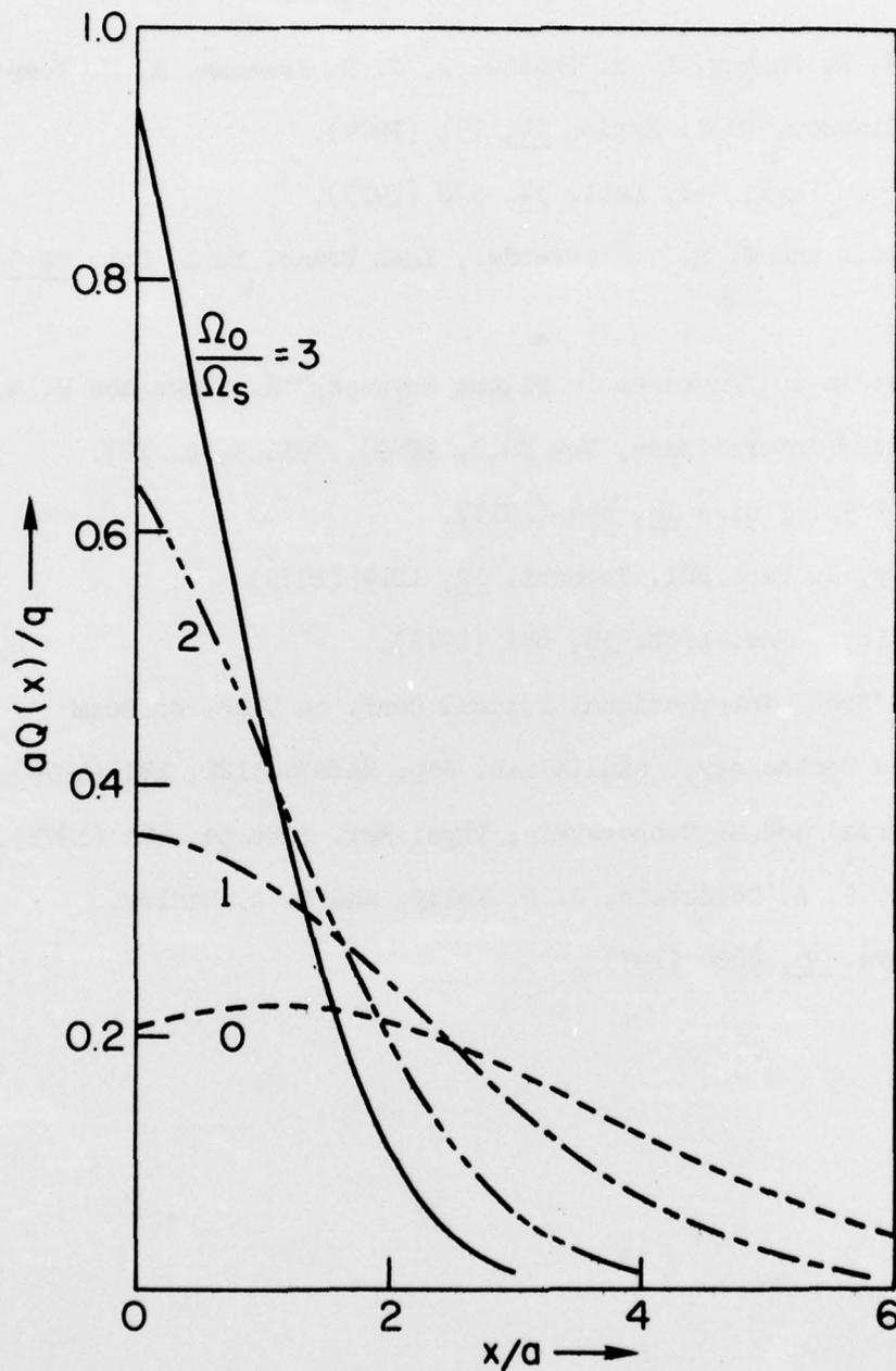
Fig. 1 — Energy deposition profiles of a 1 MeV electron beam incident on a gold plasma slab for various values of transverse magnetic-field strength. The quantity  $q$  is the integral of  $Q$  over  $x$ .
