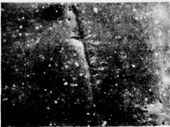
Figure 13. Surface Topography of Polished SiC Rough Lapped Balls (B2 - B4) Using Abundant Slurry.
