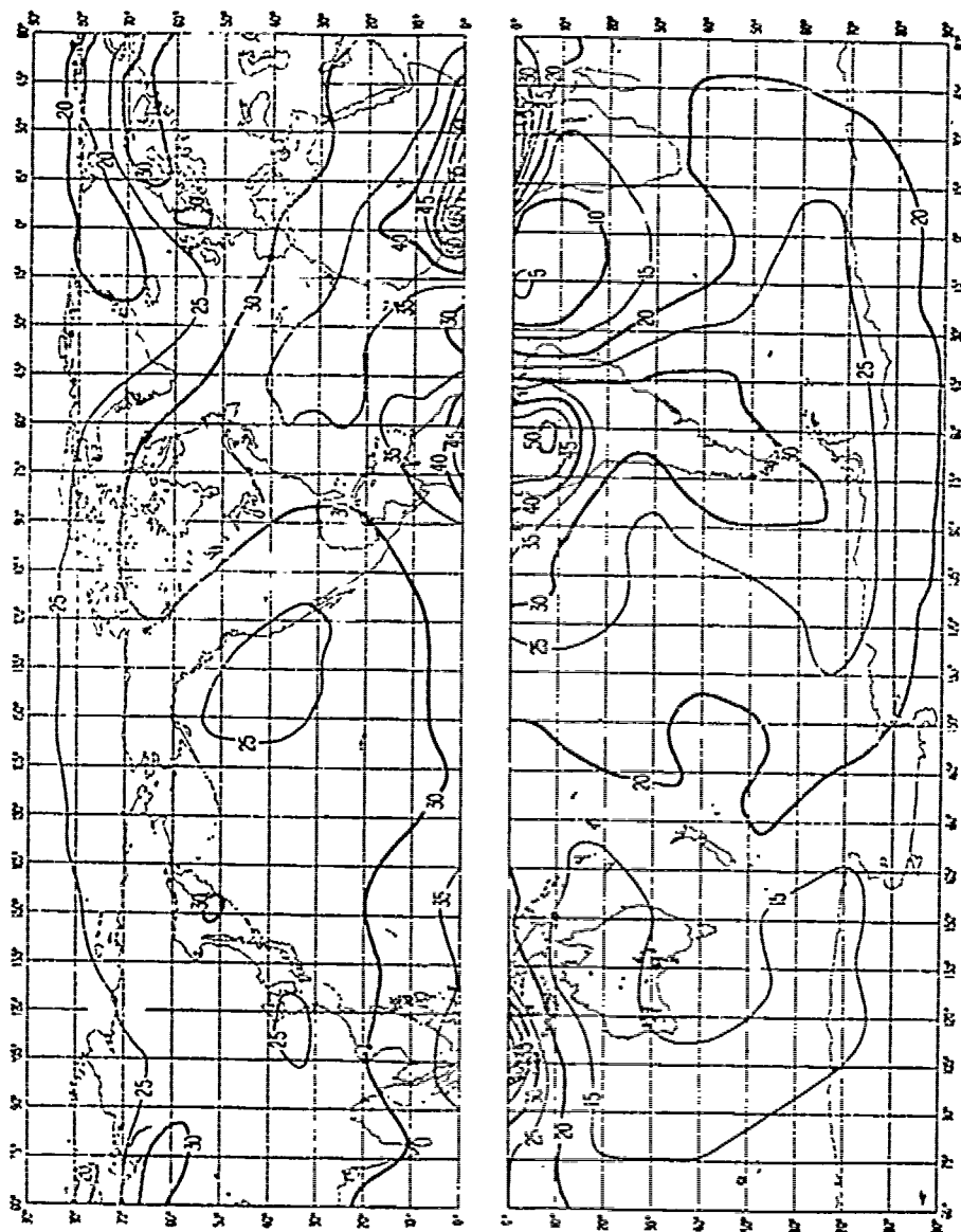
Expected values of atmospheric radio noise, F_{min} , (db above kT_{b0} at 1 Mc/s) (Winter: 0800-1200 h.)
