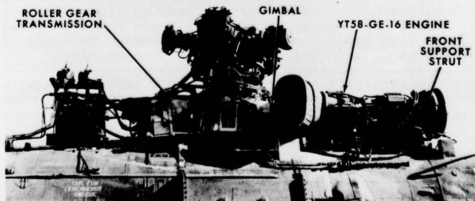
Figure 29. Engine/Transmission Installation on Tiedown Test Aircraft.
