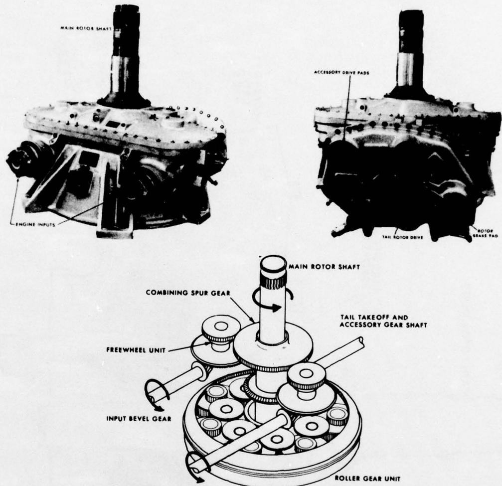
Figure 6. S-61 Roller Gear Transmission, Schematic.
