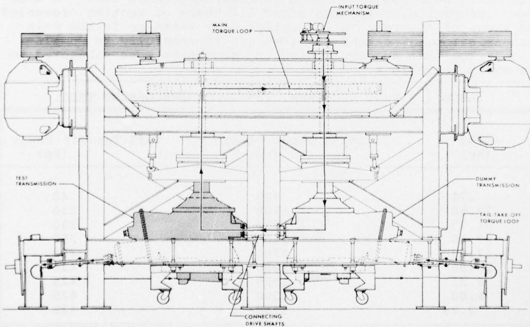
Figure 25. Roller Gear Transmission Bench Test Facility.
