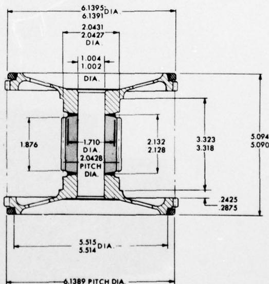
Figure 12. First-Row Pinion, Longitudinal Weld Configuration.
