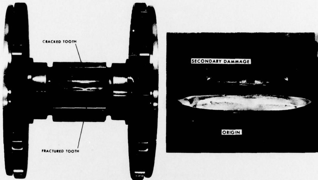
Figure 31. First-Row Pinion Tooth Fracture During R&M Test.
