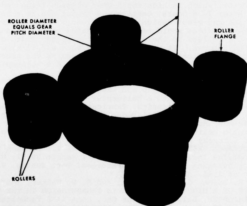
Figure 1. Roller Gear Component Concept.
