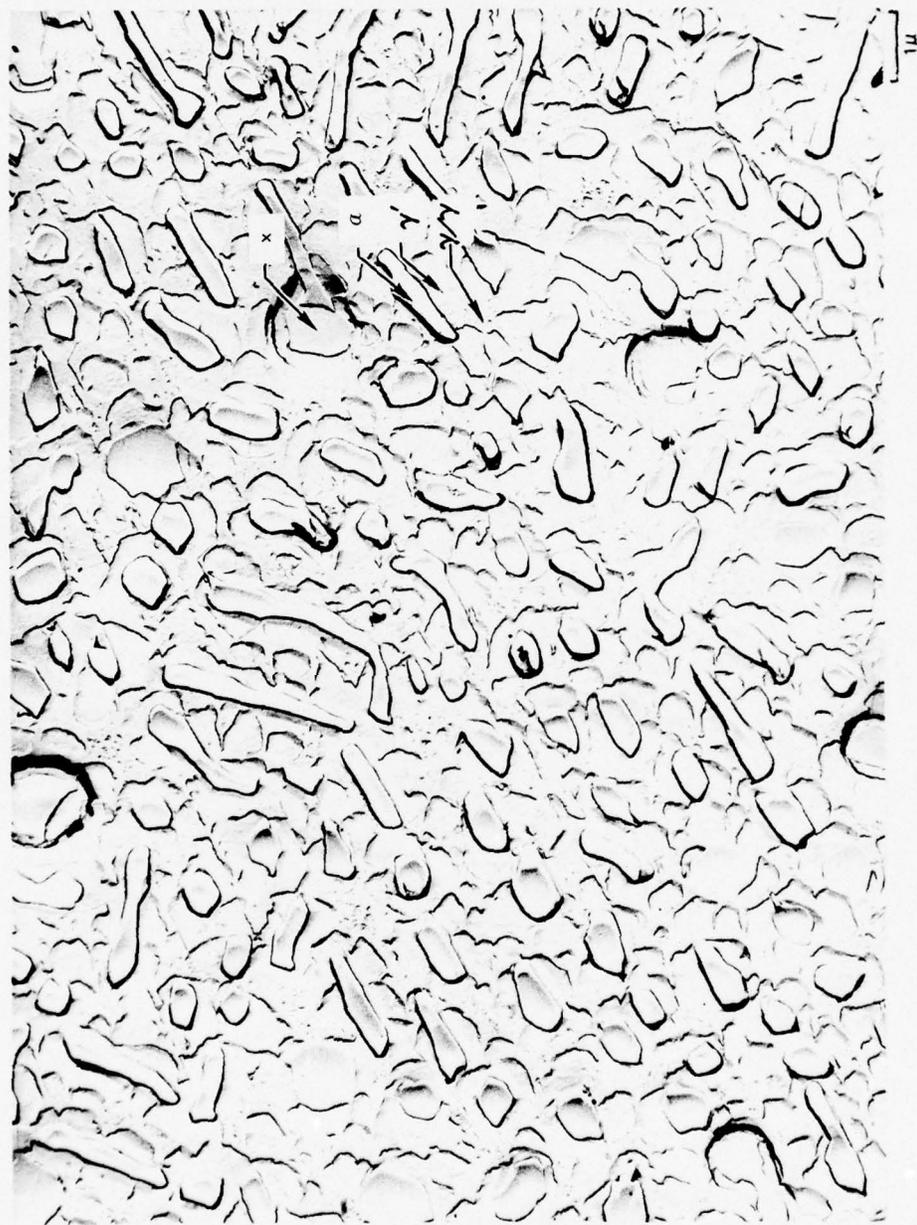
ELECTRON TRANSMISSION MICROGRAPH OF TRANSVERSE SECTION OF Ni-32 w/o Mo
