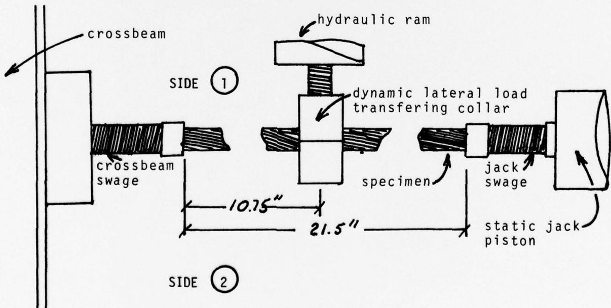
Figure 5. Test specimen set-up (dynamic lateral load)
