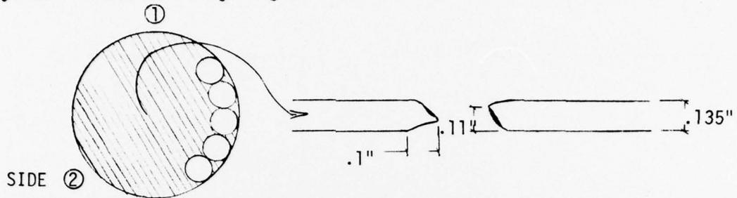
Moderate straining occurred at the crossbeam swage indicating that this region was probably approaching failure at 4300 cycles. Abrasion was high on second layer (12 wires) at midspan and at both swages.
