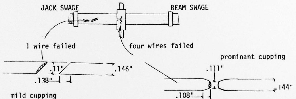
Abrasion occurred between outer (18 wire) and first (12 wire) layers. At cable midspan abrasion was high and decreased to low at swages.
