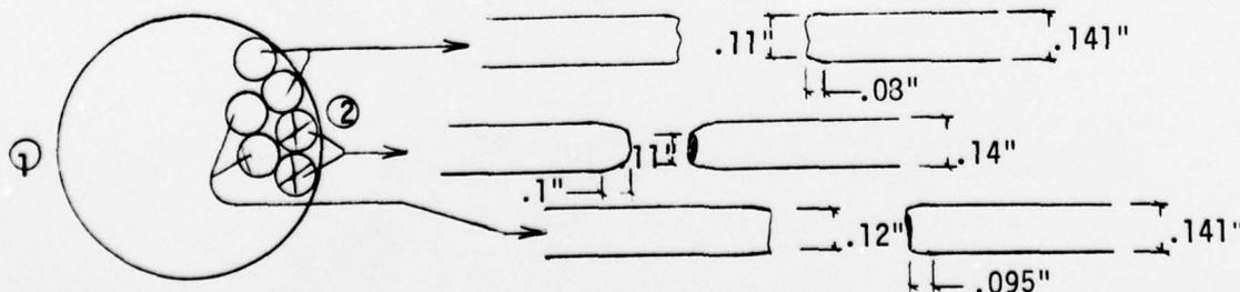
Failure here was probably due to swage abrasion of wires on specimen outer layer. Ultimate failure followed rapidly with only five strands remaining at crossbeam swage. Four additional strands broke at the jack swage as noted above. Failed wires at crossbeam swage showed signs of bending
