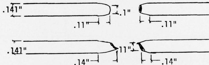
Abrasion was highest at midspan on second layer (12 wires) decreasing slightly at swages. In general, degree of abrasion was moderately high.
