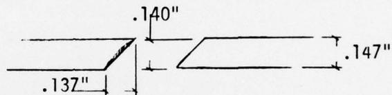
Failure plane was about 45° with very little local strain. However, entire outer layer of cable showed strain in excess of other layers of about .047".
