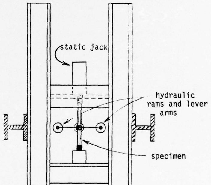
Figure 7. Schematic for torsion test
