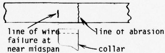
30 wires failed at swage with average depth of failure point in swage of .09 inch. All outer layer wires that failed here were at swage surface while inner wires failed at depths as great as .39 inch. Abrasion was moderate on second layer (12 wires) at swage and heaviest on second layer at about cable midspan.
