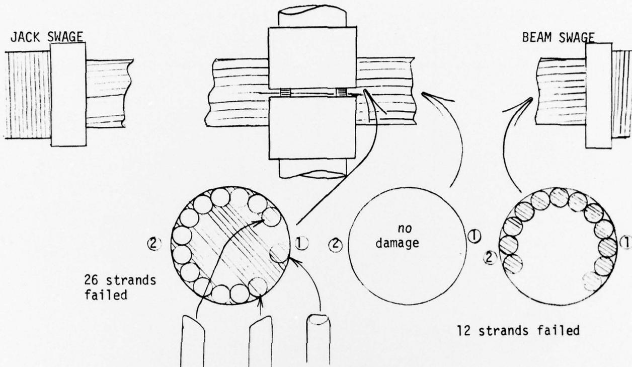
Primary failure occurred at point where 12 strands cable entered collar.
