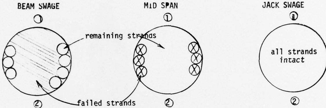
It is not known which wires failed first. However, it is likely that midspan failure occurred first due to high abrasion from collar and that swage failure followed due to excessive axial load on remaining strands and large lateral deflection of cable at midspan with ensuing high end moments.
