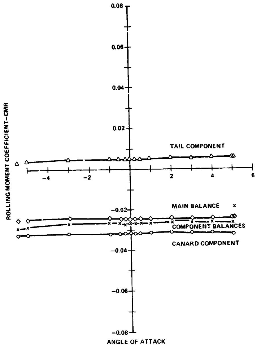
Figure 44. Component rolling moment coefficient,
