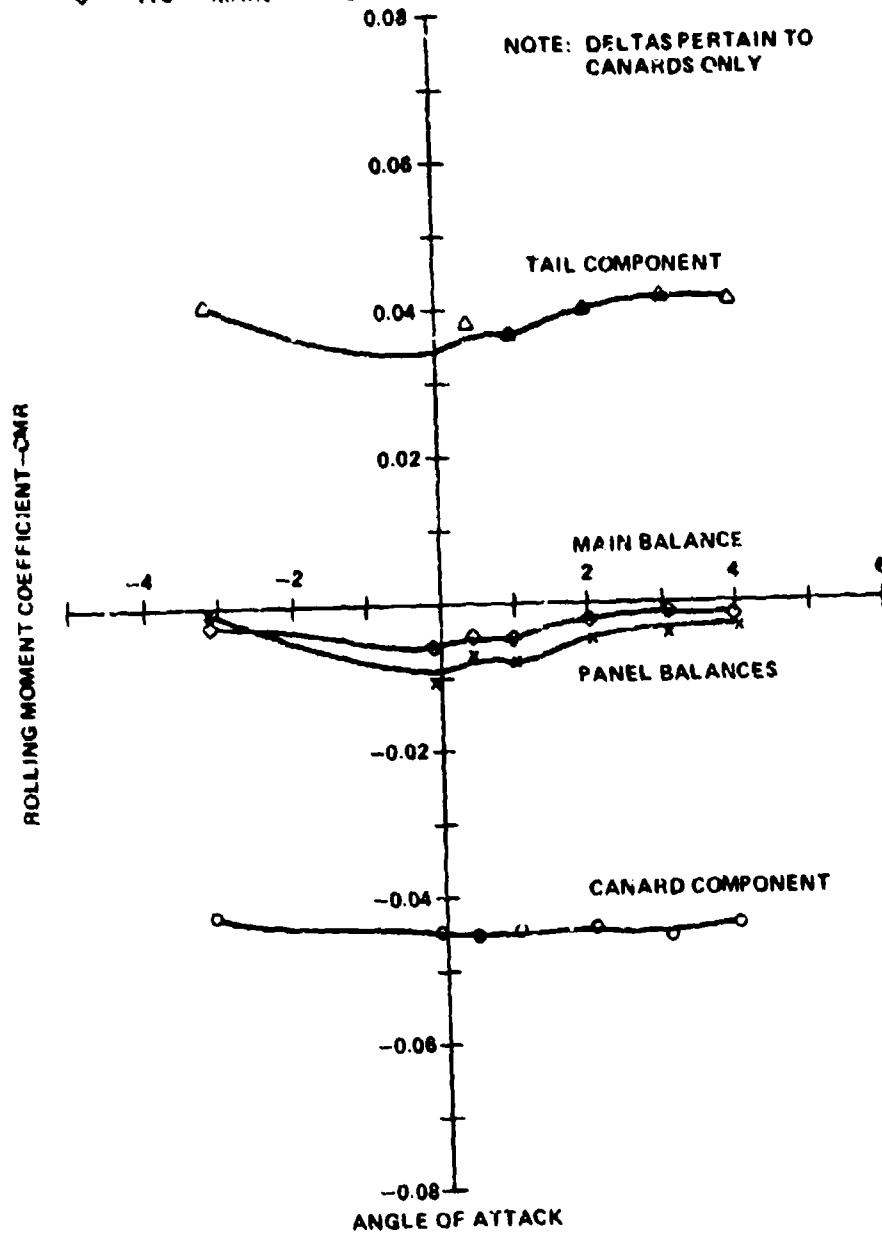
Figure 7. Component rolling moment coefficient,
