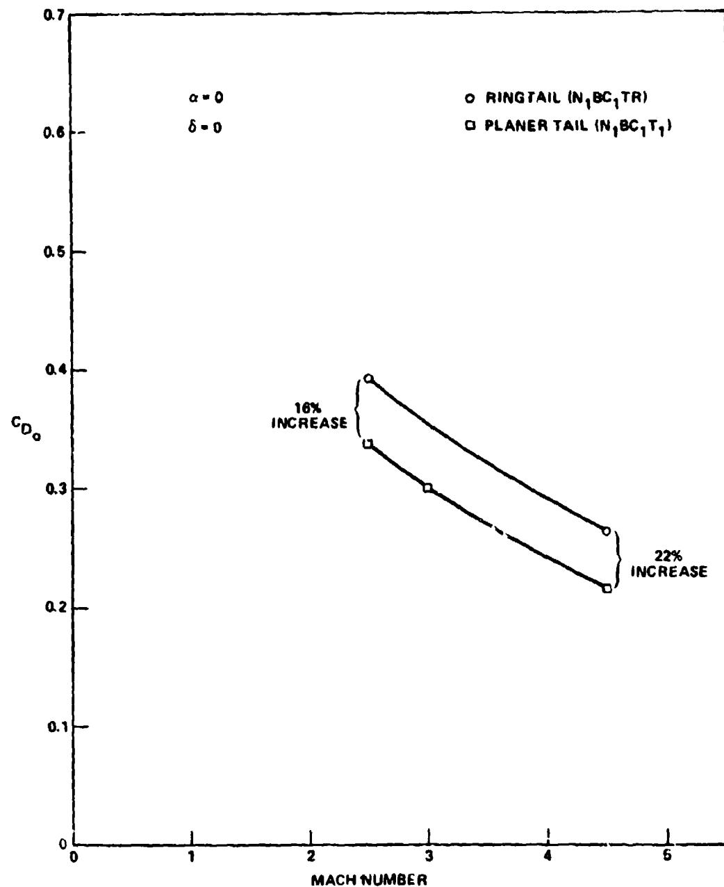
Figure 50. Change in drag due to ring tail.
