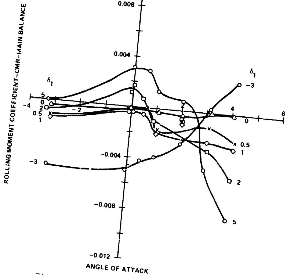
Figure 31. Total rolling moment coefficient,
