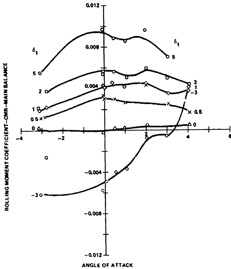
Figure 19. Total rolling moment coefficient,
