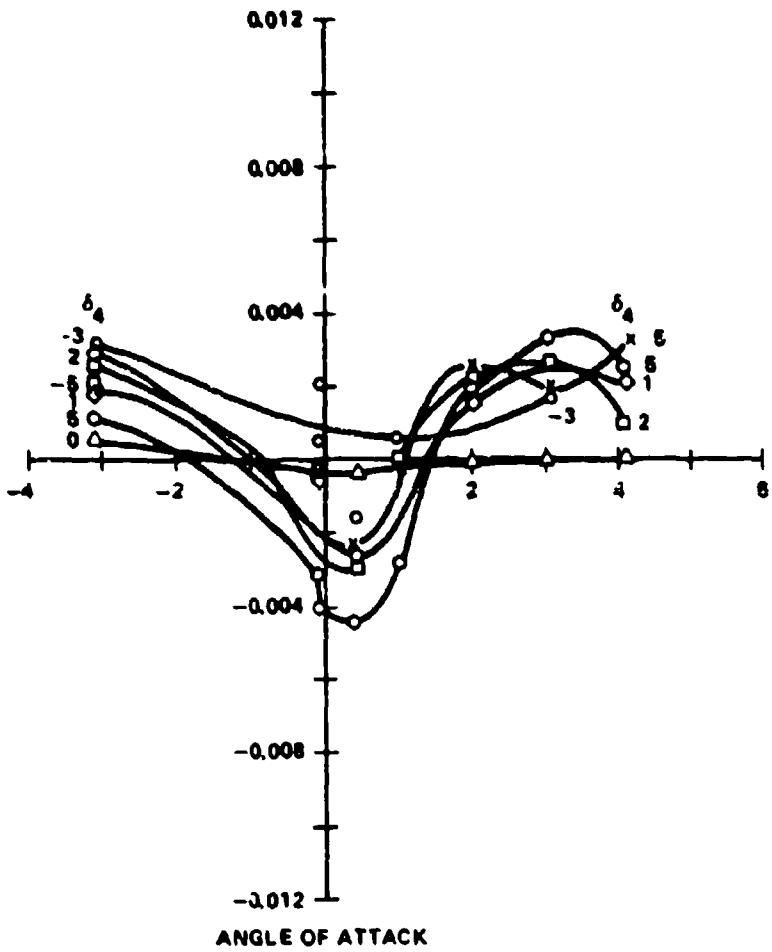
Figure 25. Total rolling moment coefficient,  $M_\infty = 0.6$ , forward canards, planar tail.
