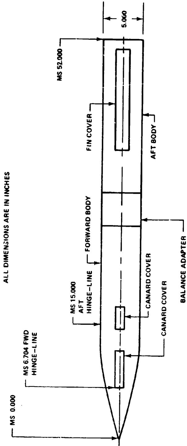
Figure 2. Sketch of model body showing hinge-line positions for canards.
