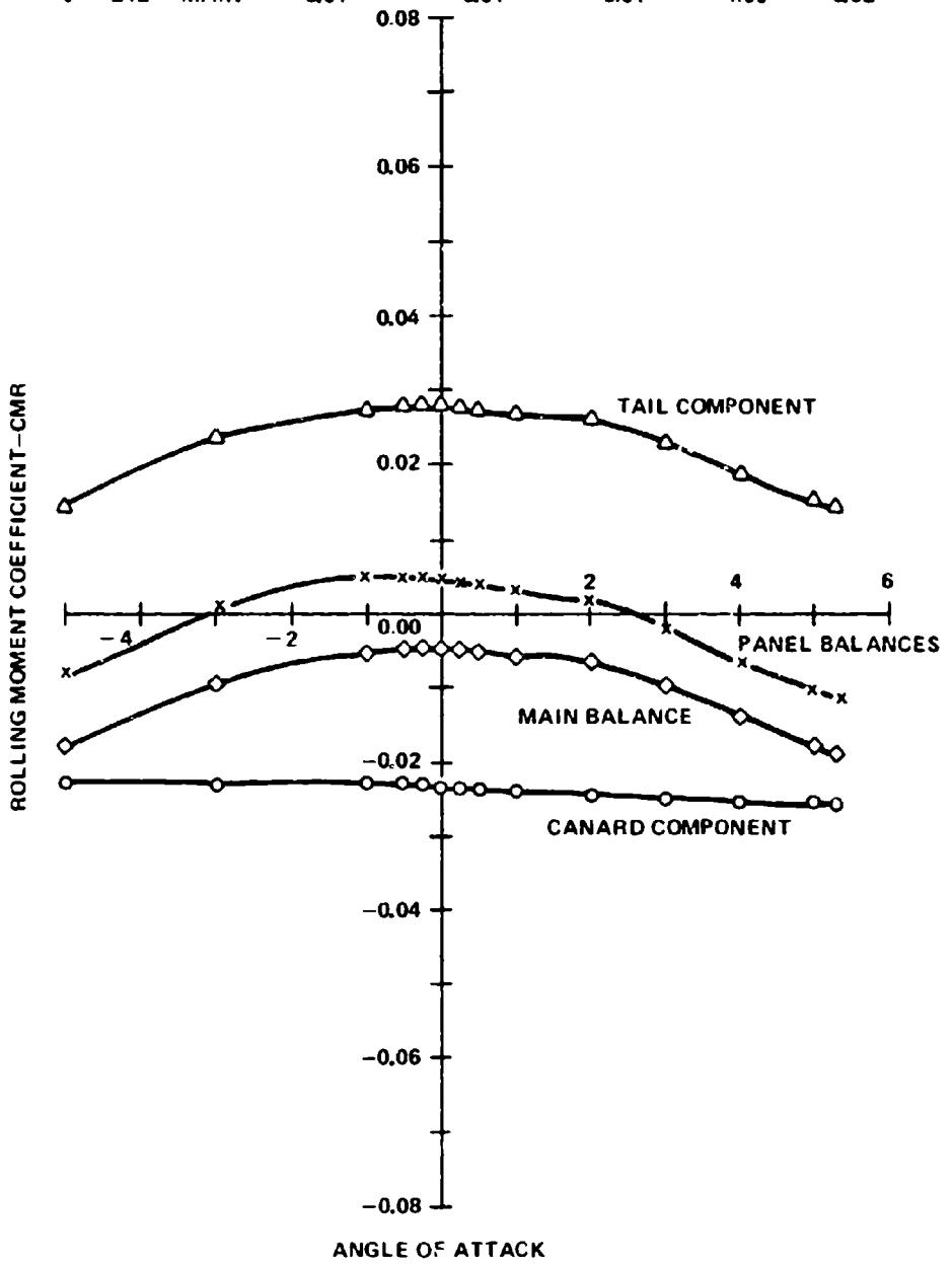
Figure 14. Component rolling moment coefficient,
