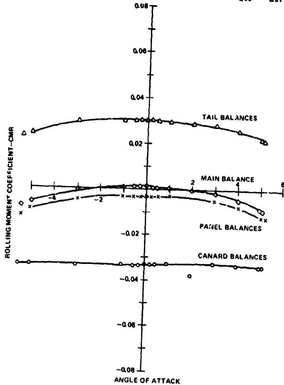
Figure 22. Component rolling moment coefficient,
