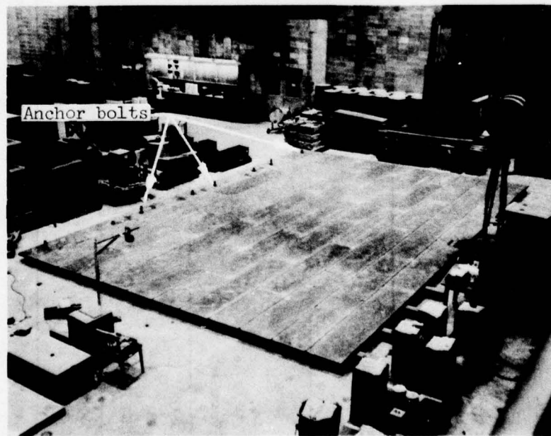
Photograph 2. Test setup for 2- by 9-ft mat (36 ft wide)
