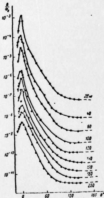
Fig. 1. Distribution of luminance  $B(\theta)$  in the light field of an isotropic source at various distances  $r$ .
