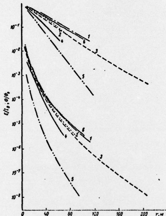
Fig. 2. Irradiance  $\frac{E(r)}{I_0}$  and flux  $\frac{\phi(r)}{\phi_0}$  through a sphere of radius  $r$  vs distance  $r$  from isotropic source.
