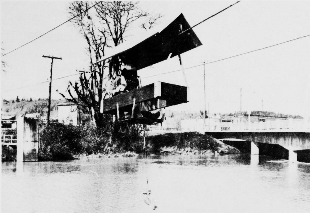
Photo IV-1. Measuring streamflow from a cableway, Long Tom River at Monroe, Oregon.
