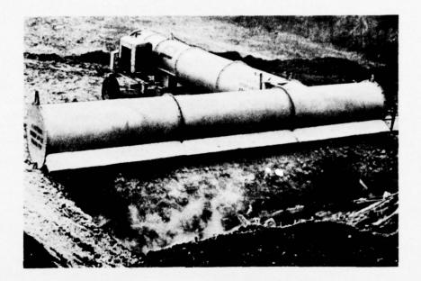
Figure 14. Earth pit for pit incineration.
