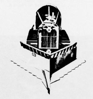
Figure 8. "V"-shaped shear blade with splitter.
