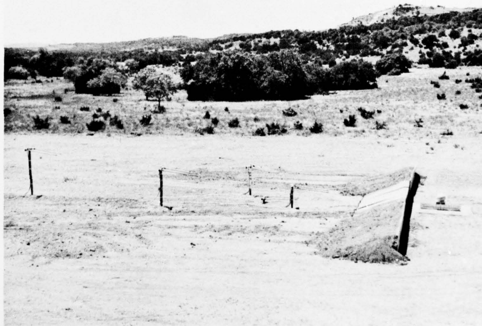
FIGURE 19. SINGLE-REVETTED, 24-IN. BARRICADE NEAR FIELD, 64-LB EXPERIMENTS
