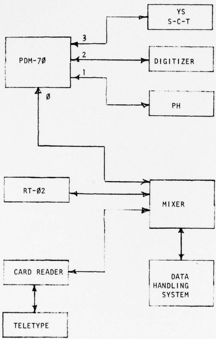
FIGURE 2 DATA HANDLING SYSTEM - AUTOMATED INSTRUMENTATION INTERCONNECTIONS
