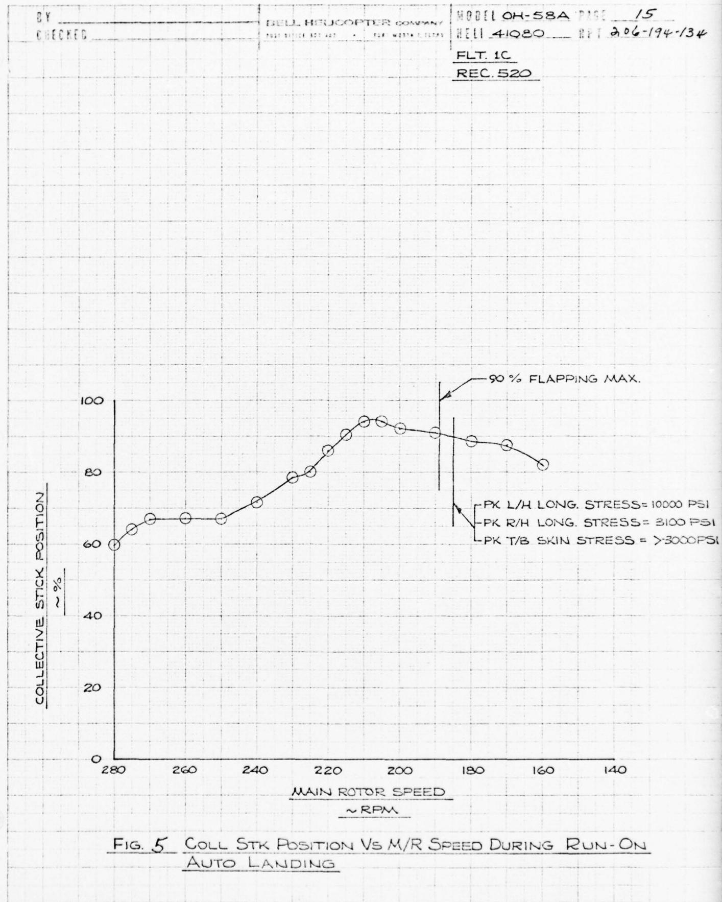
FIG. 5 COLL STK POSITION VS M/R SPEED DURING RUN-ON
