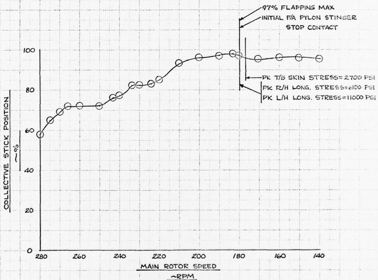
FIG. 1 COLL STK POSITION VS. M/R SPEED DURING RUN-ON
