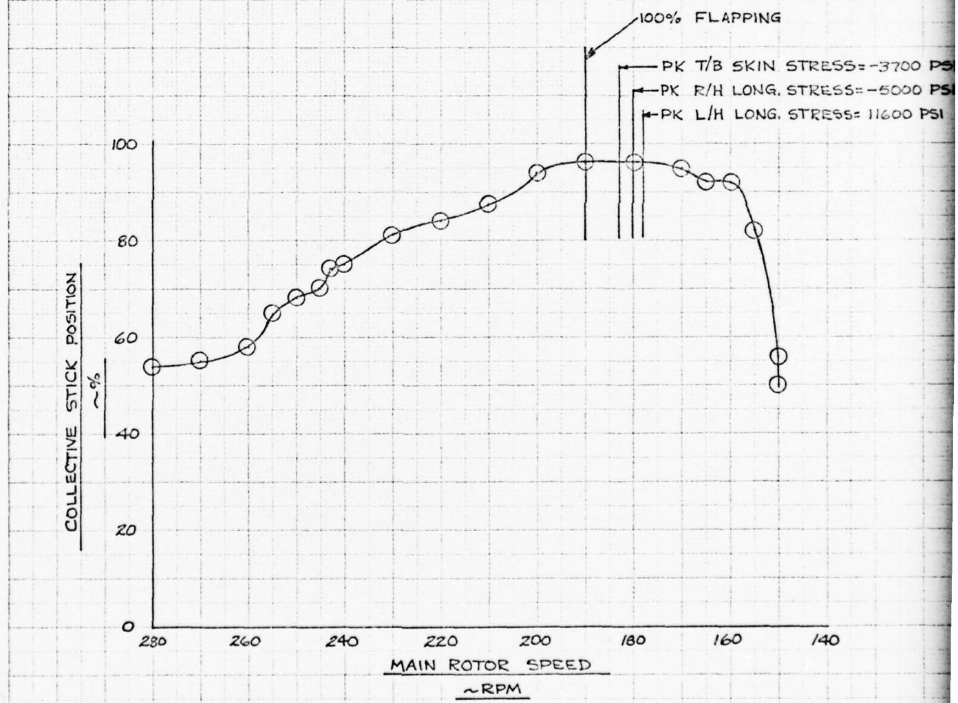
FIG. 4 COLL STK POSITION Vs. M/R SPEED DURING RUN-ON
