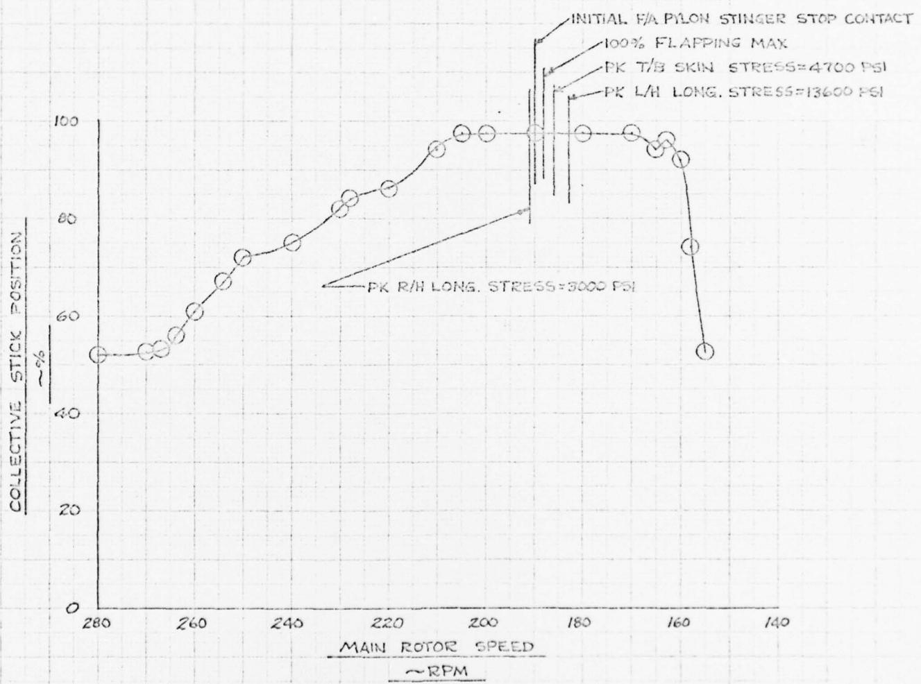
Fig. 16 COLL. STK. POSITION VS. M/R SPEED DURING RUN-ON
