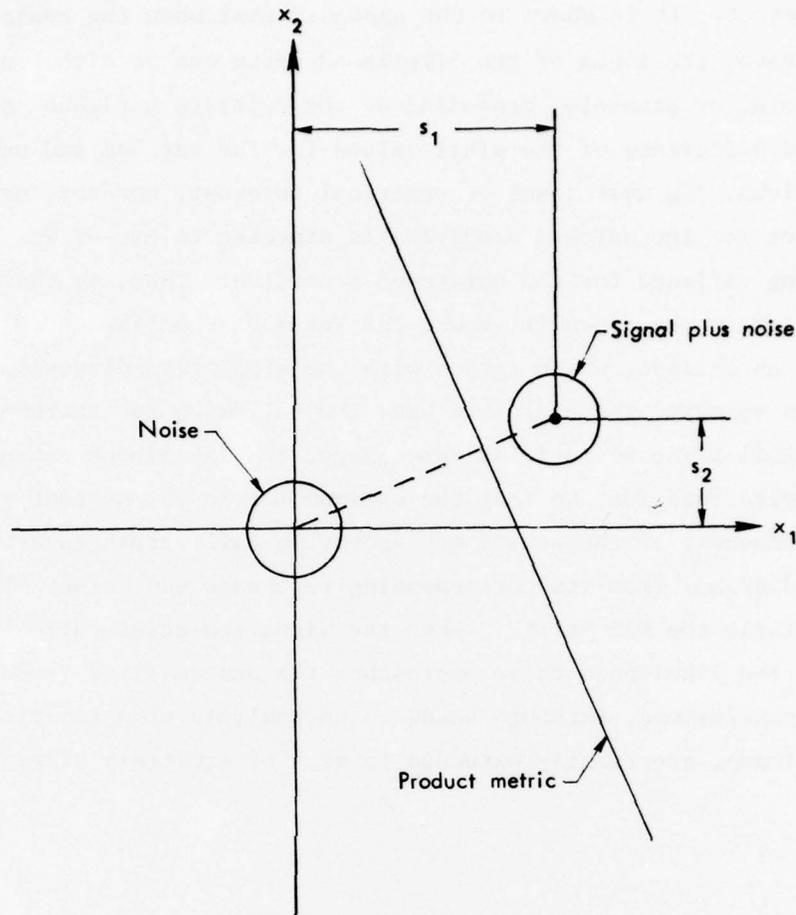
Fig. 2—Schematic representation of the signal-detection problem
