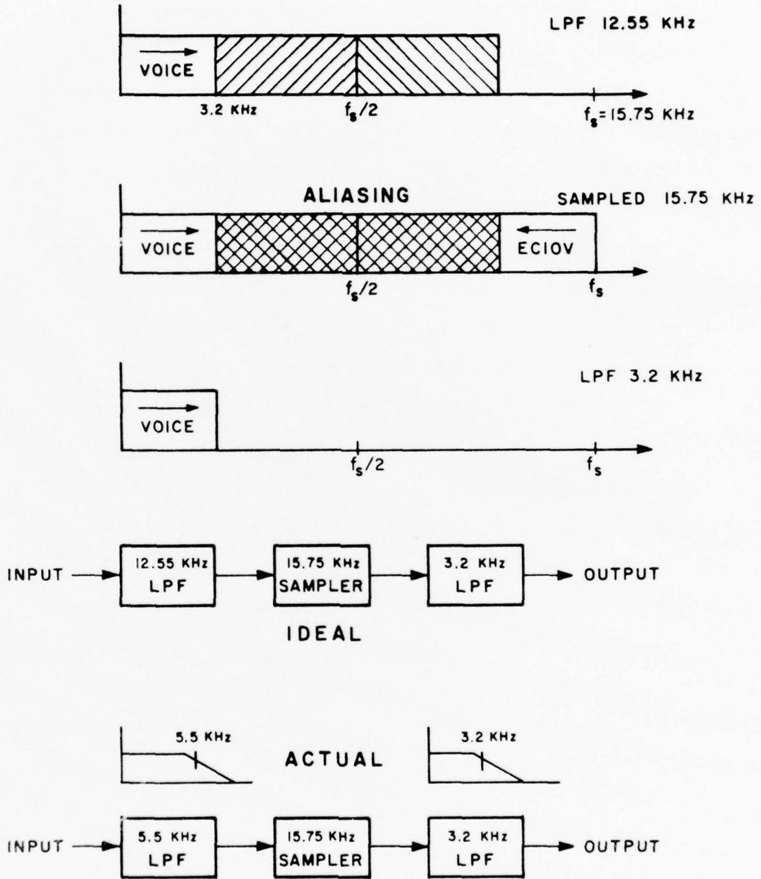
Figure 12. Audio Filtering
