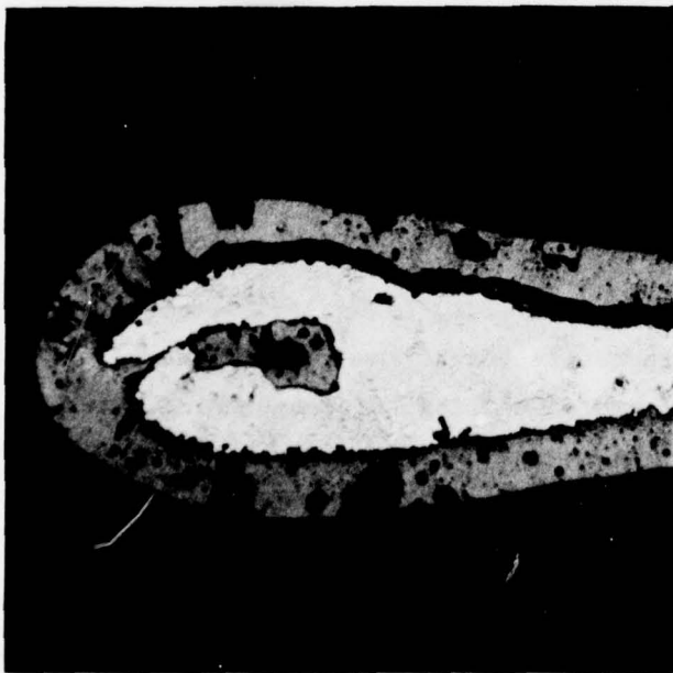
Fig. 3c. Ni-8Si-12Nb, Oxidized 51 hrs at 1150°C X100
