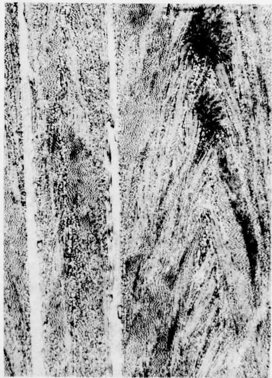
Fig. 1d. Ni-19.1Cr-16Zr X500 Etched in 96H 2 O 2 , 2HNO 3 , 2HF
