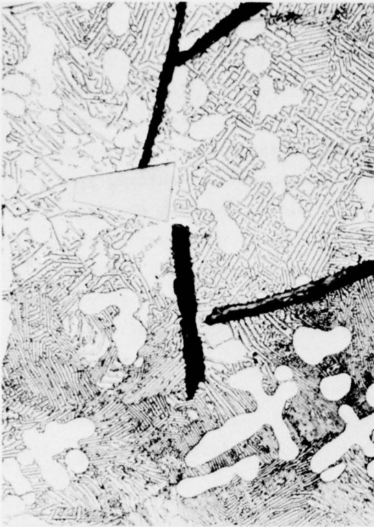
Fig. 1a. Ni-5C-20Zr X500 Etched in 65H 2 O, 22H 2 O 2 , 13HCl(vol%)
