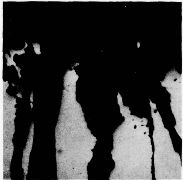
Fig. 3b. Ni-7Si-8Zr, Oxidized 24 hrs at 1150°C X500
