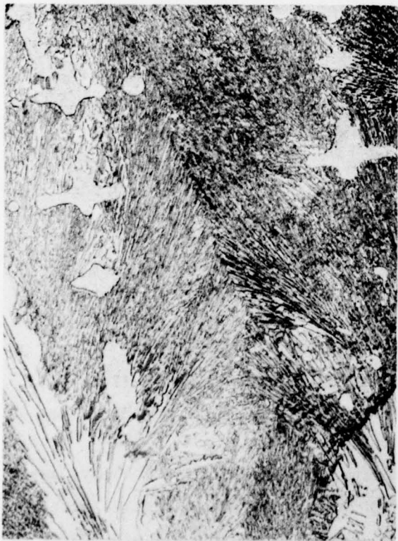
Fig. 1c. Ni-9Si-17Nb X500 Etched in 65H 2 O, 22H 2 O 2 , 13HCl
