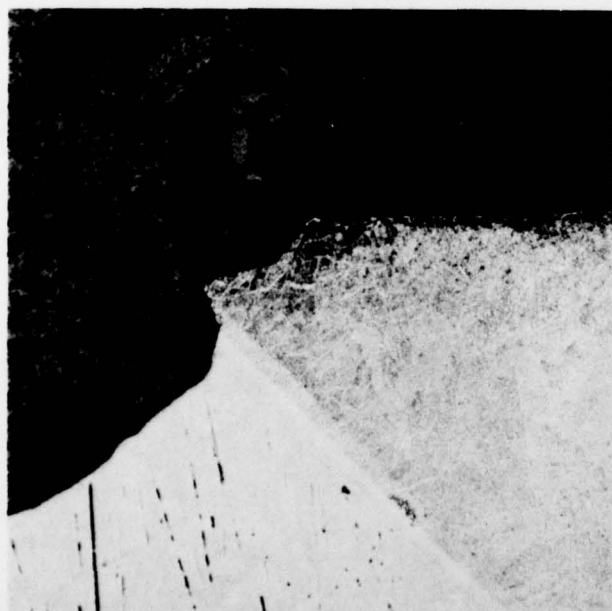
Fig. 8c. Co-5Al-23Nb, Oxidized 3 hrs at 1150°C
