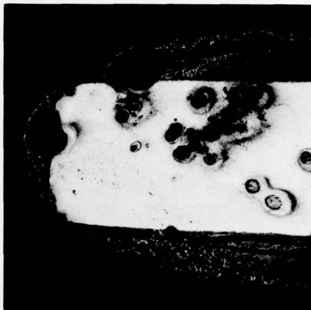
Fig. 8b. Fe-6.5Si-8.5Nb, Oxidized 15 mins. at 1150°C
