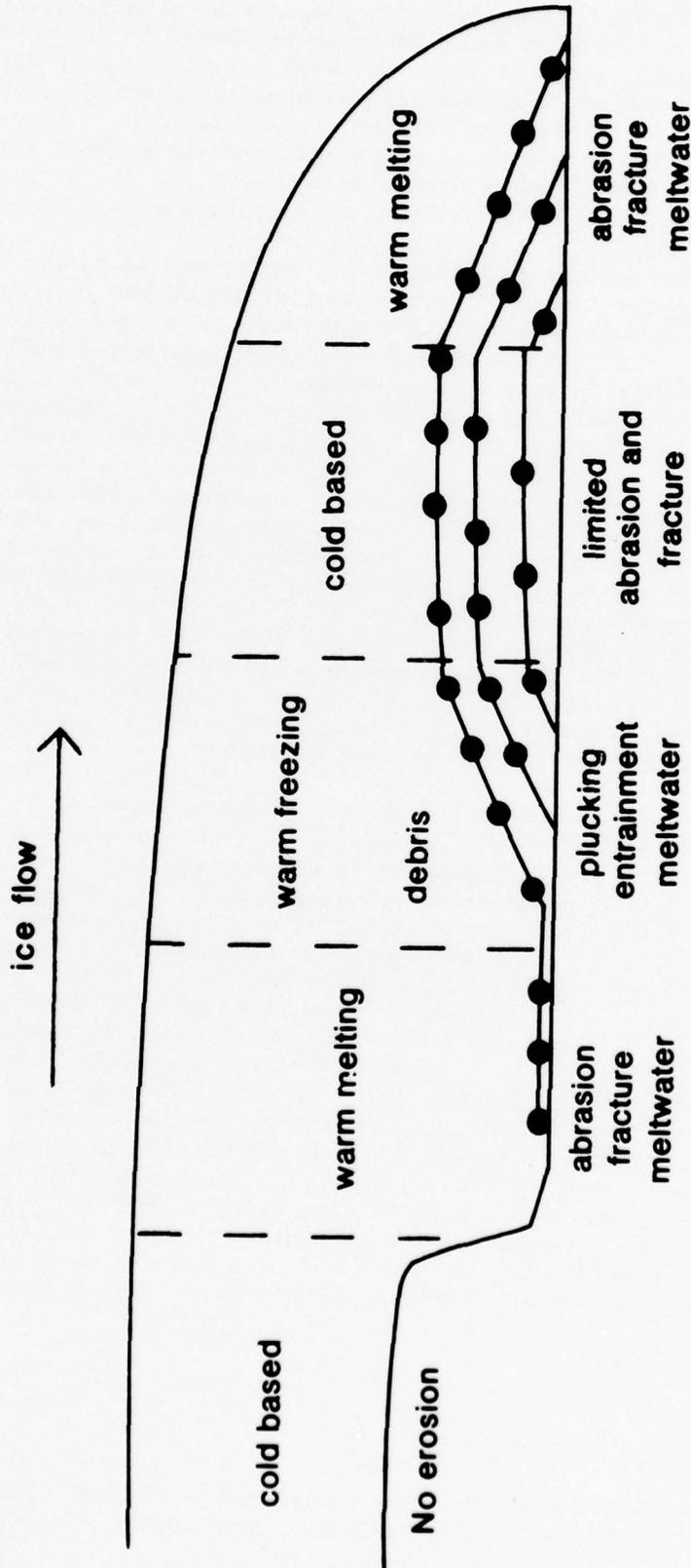
Figure 20. Idealised model of the relationship between processes of glacial erosion and the basal thermal regime of an ice sheet.
