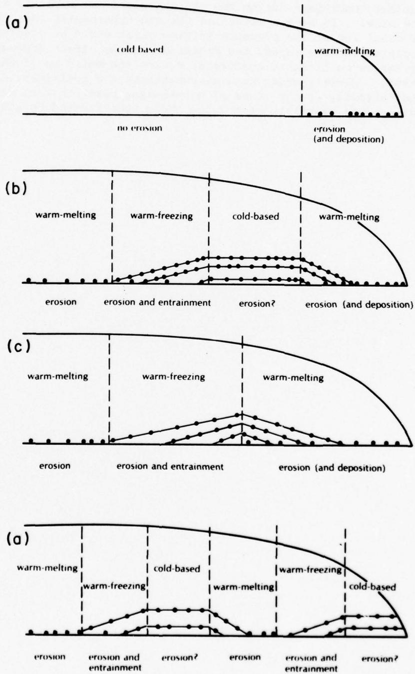
Figure 12. Various sequences of basal thermal regime and associated erosional processes encountered beneath the Laurentide ice sheet at its maximum.
