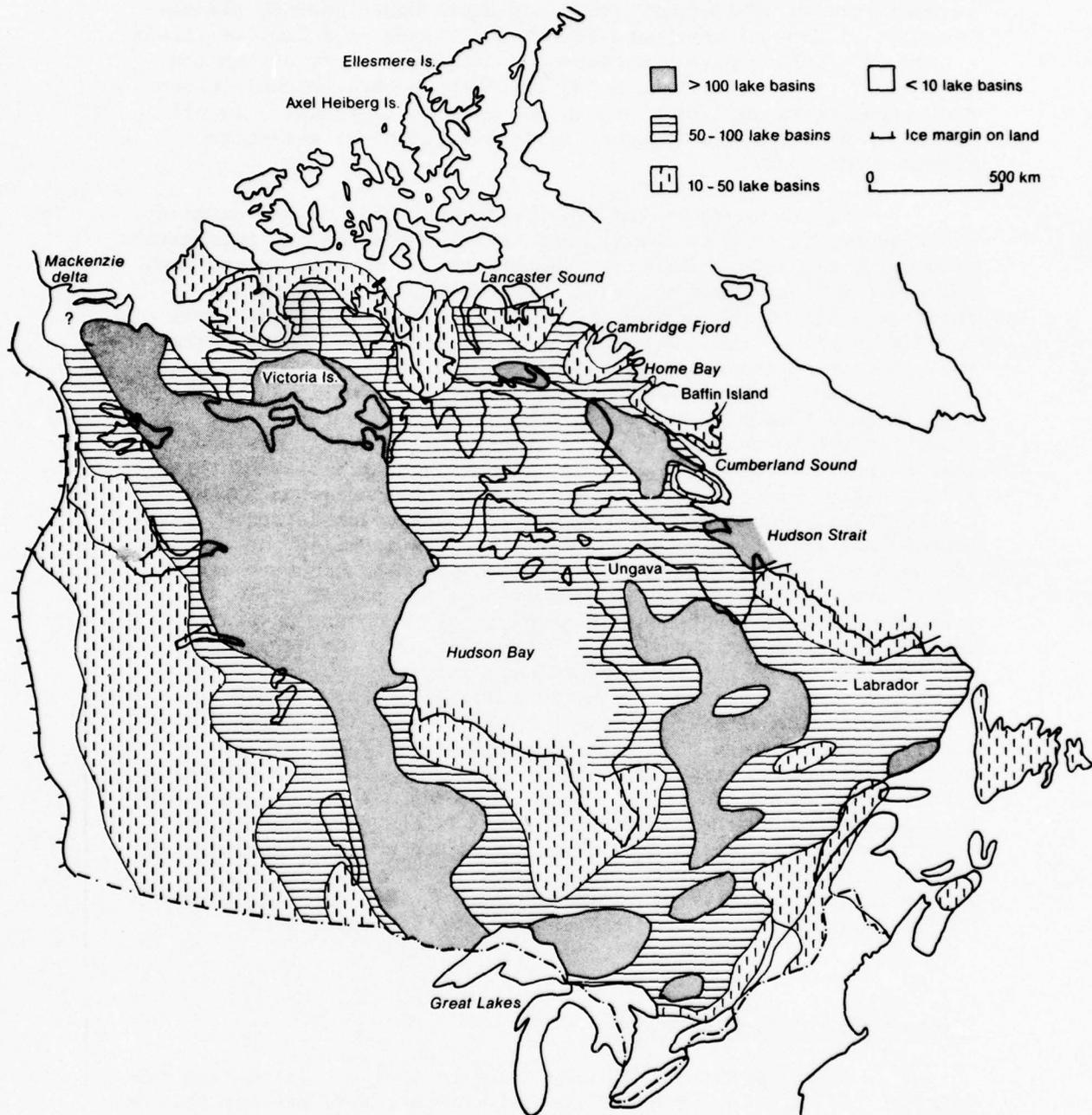
Figure 19. The density of lake basins (0.5 to 2.0 km. in diameter) in unit areas of 400 km.<sup>2</sup> in Canada. The data was obtained by sampling from flat areas on topographic maps at a scale of 1:500,000. Lake basin density at this scale is thought to be a measure of the intensity of glacial erosion.
