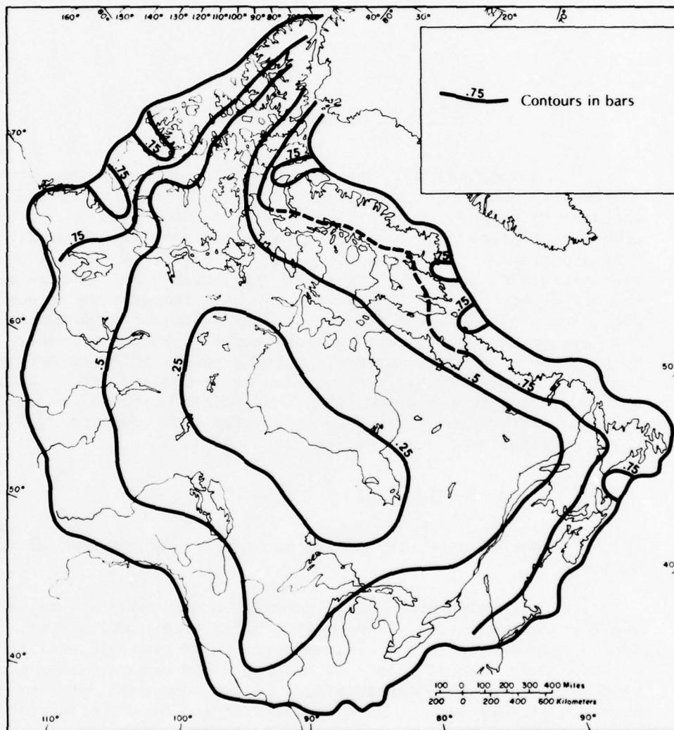
Figure 9. Calculated basal shear stresses beneath the Laurentide ice sheet at its maximum.
