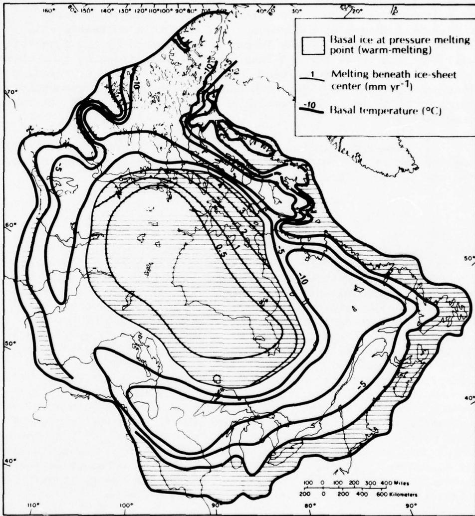
Figure 10. Calculated basal temperatures and zones of basal melting beneath the Laurentide ice sheet at its maximum.
