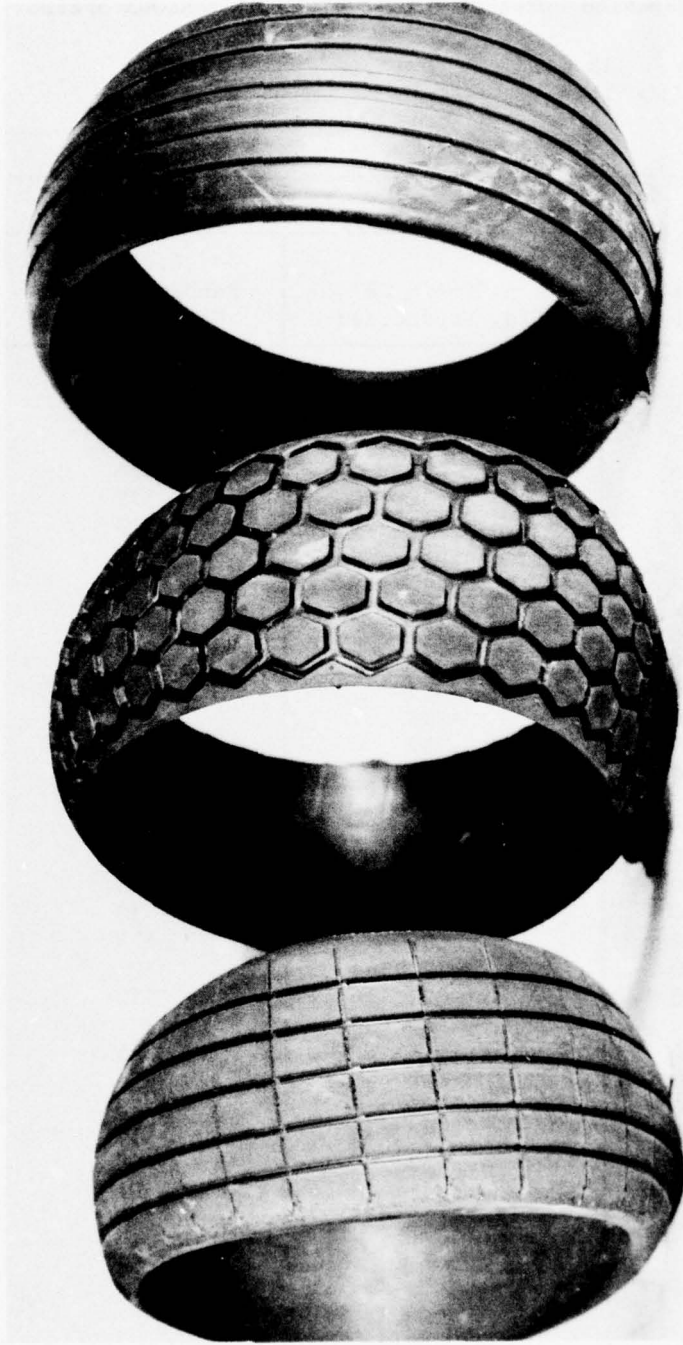
Figure 8. Replaceable Belts of Various Tread Designs: The Circumferentially and Laterally Grooved, the Knobby, and the Circumferentially Grooved Replaceable Tread Belts
