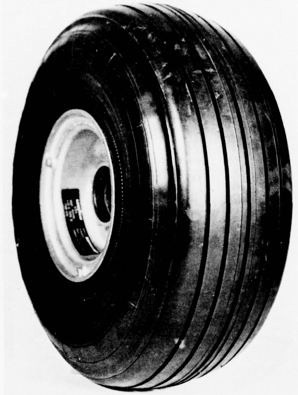
Figure 7. 6.00-6 Rubber Carcass with Mounted Circumferentially Grooved Tread Belt - The Replaceable Tread Tire
