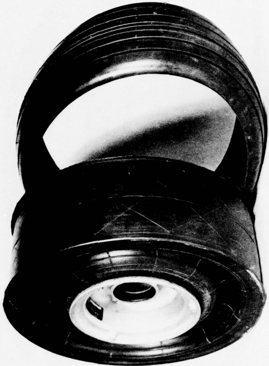
Figure 6. 6.00-6 Rubber Carcass with Dismounted Circumferentially Grooved Tread Belt
