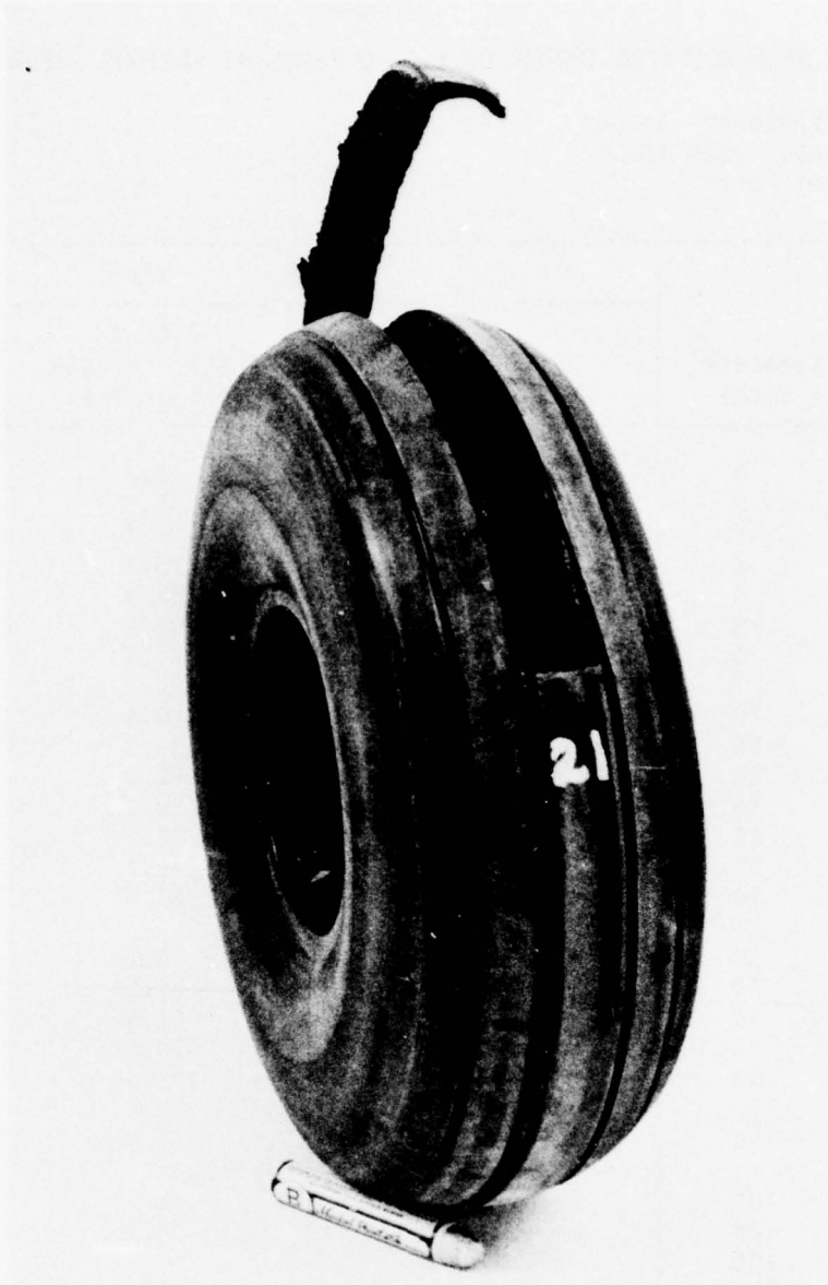
Figure 9. Cast Tire: Failure Occurred During Cornering Tests
