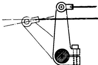
Fig. 7.3-14 Attachment of a cable to a lever
