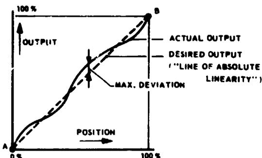
Fig. 3.2-5 Absolute linearity in a linear potentiometer
