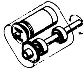
Fig. 7.2-4 Coupling of the intermediate shaft by gears
