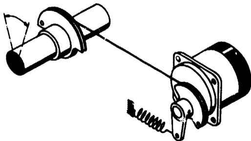
Fig. 7.3-11 Simple wire coupling with a single wire
