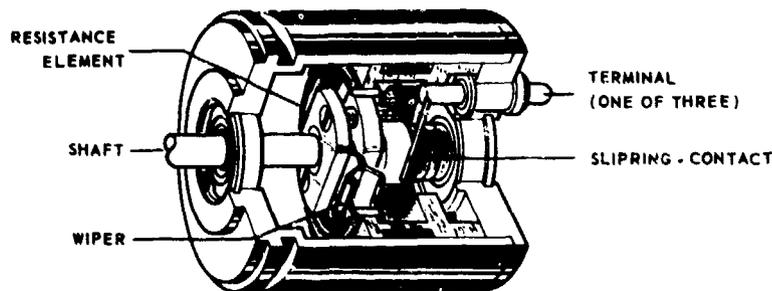
Fig. 3.2-2 Construction of a single turn wire-wound potentiometer.
