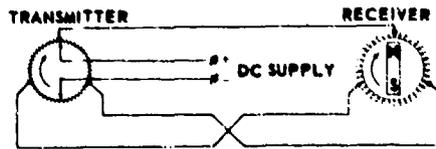
Fig. 4.2-13 Principle of the DC synchronous system
