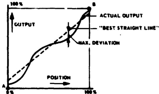
Fig. 3.2-7 Independent linearity in a linear potentiometer
