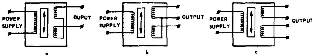
Fig. 5.2-4 Output configurations of variable differential transformer
