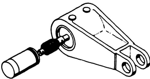
Fig. 7.3-1 Directly coupled transducer using a flexible coupling
