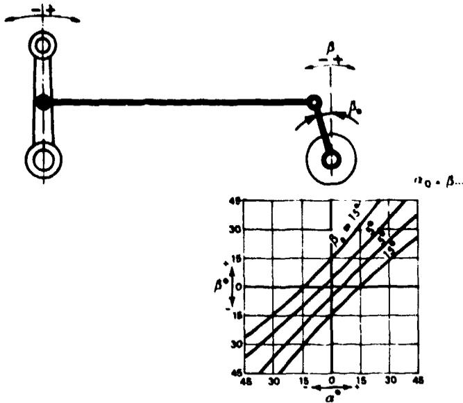
Fig. 7.3-4 Linearity errors due to non-parallel levers
