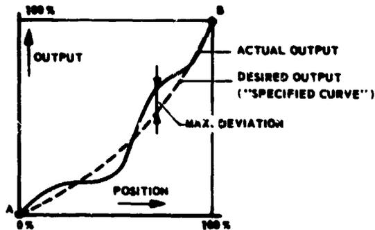
Fig. 3.2-6 Absolute conformity in a non-linear potentiometer
