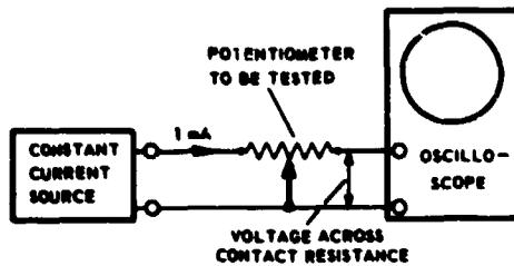
Fig. 3-2-13 ENR test for rotary wire potentiometers
