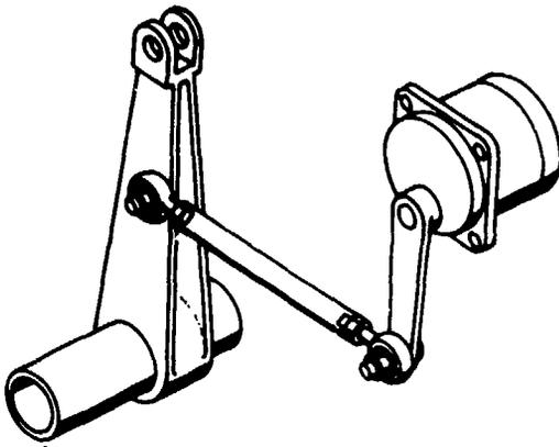
Fig. 7.3-3 Lever coupling
