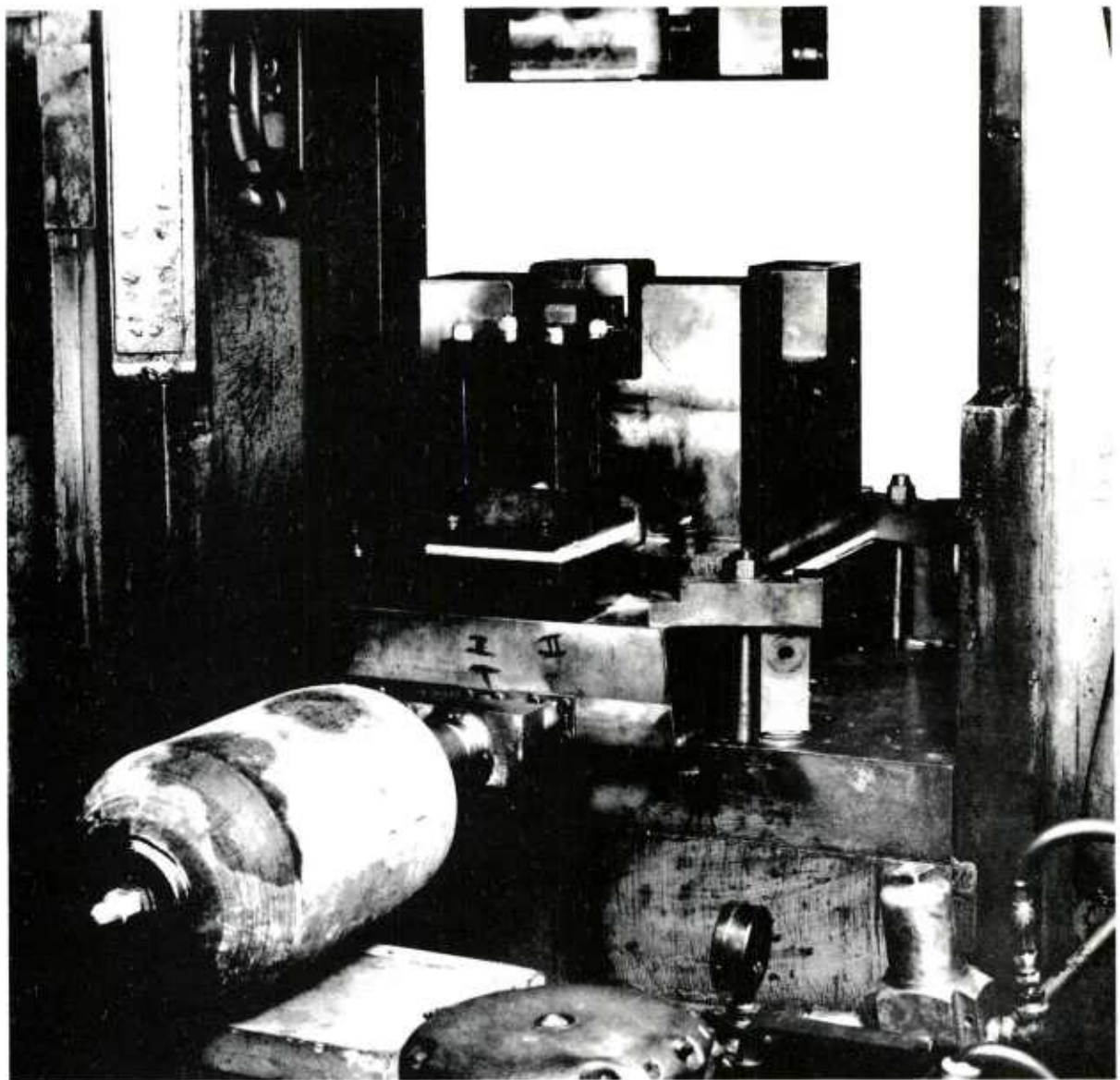
Figure 14. Hammer Forging Die Set Installed in a Hydraulic Press for Initial Tryout.
