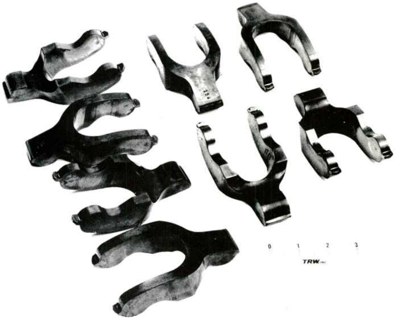
Figure 17. As-Forged Accelerators Produced from Sintered P/M Preforms.
