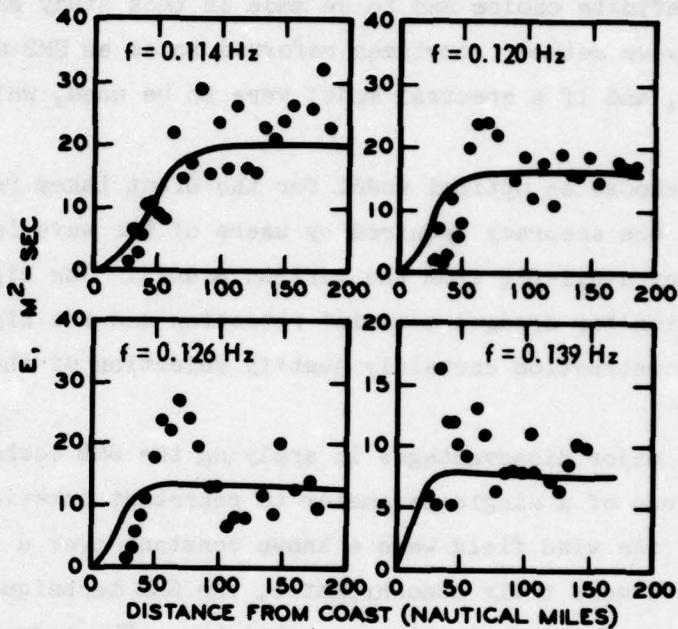
Figure 14. Growth of frequency components of waves for an offshore wind of 30 knots (after Barnett<sup>30</sup>)
