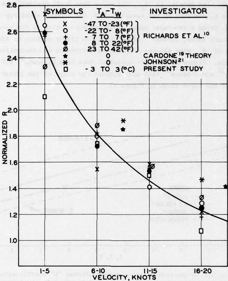
Figure 13. Velocity-dependent behavior of the ratio of anemometer-level wind speeds ( $V$ ) to geostrophic wind speeds ( $G$ ). Values for  $V/G$  have been normalized to neutral conditions assuming a value of  $V/G$  for land of 0.45
