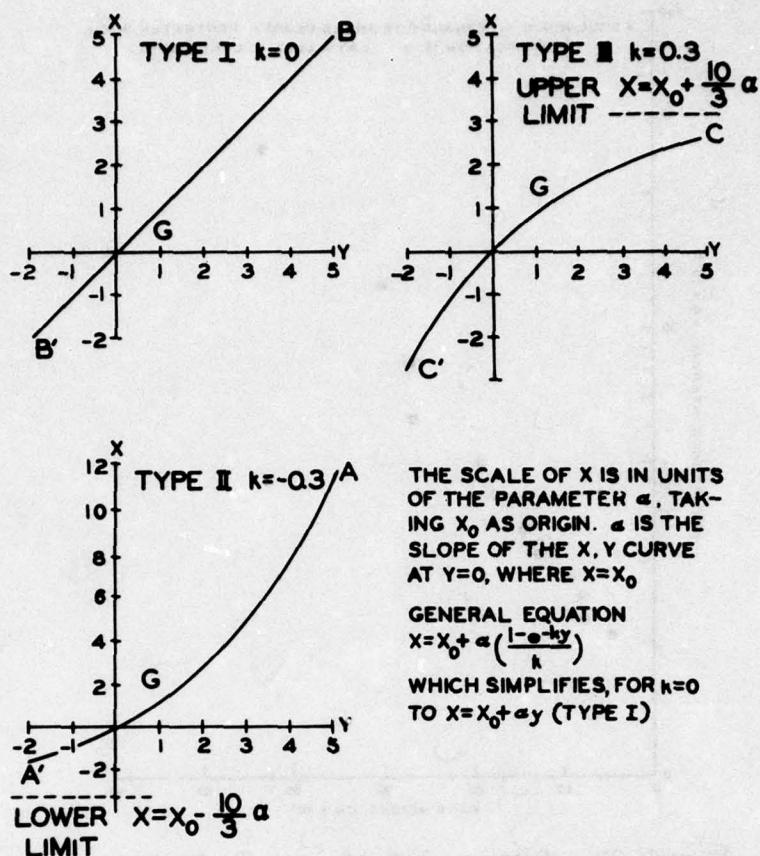
Figure 19. Schematic representation of the three Fisher-Tippett asymptotic distributions on x-y diagrams (after Jenkinson<sup>44</sup>)
