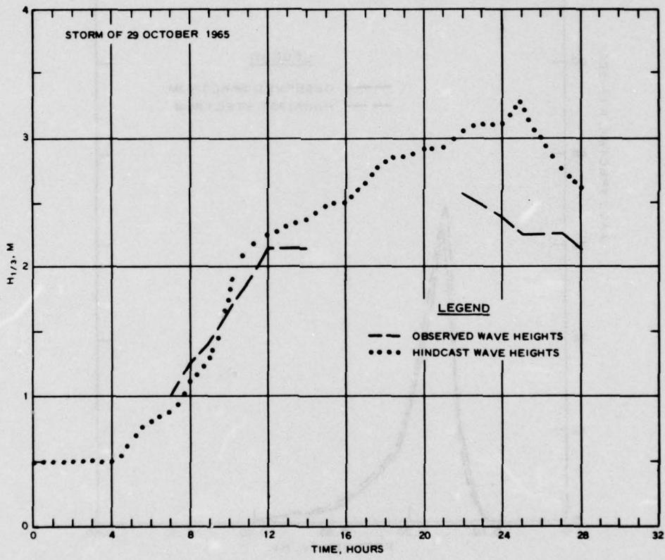
Figure 16. Comparison of time series of significant wave heights observed at Muskegon for storm of 29 October 1965 and wave heights hindcast by numerical model for same storm
