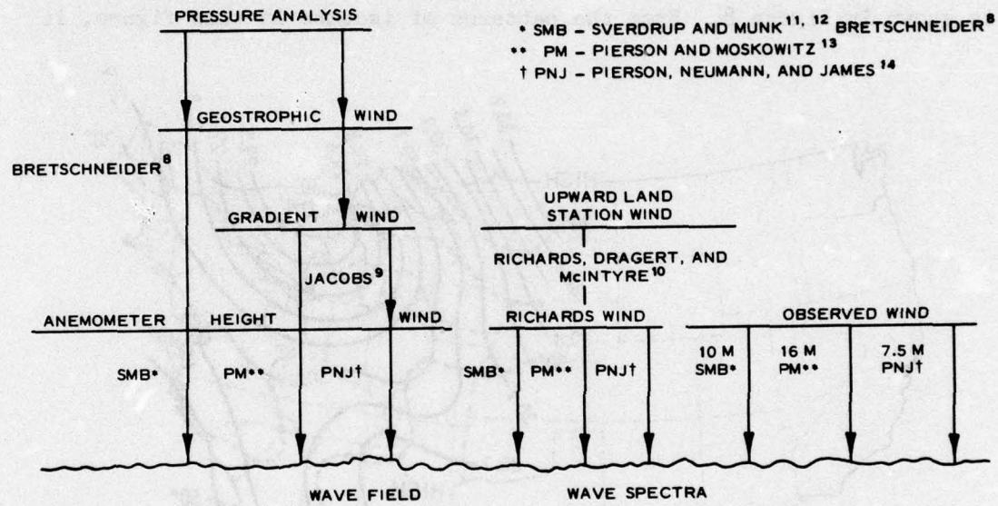
Figure 7. Schematic diagram of wind techniques investigated by Cole<sup>7</sup>
