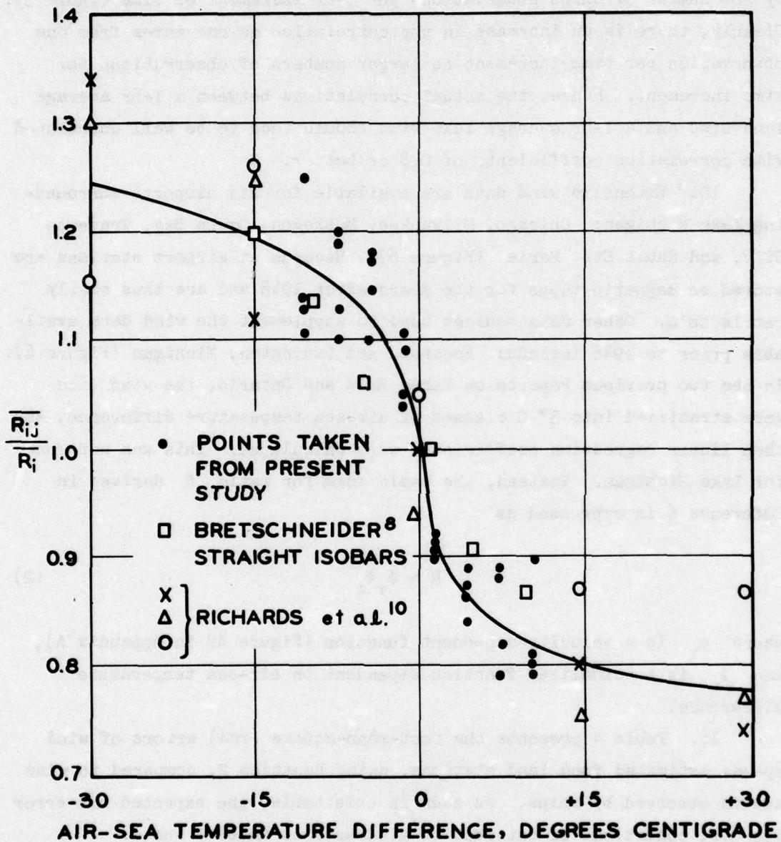
Figure 11. Comparison of empirical results of Richards et al.,<sup>10</sup> Bretschneider,<sup>8</sup> and the present study. The data of Richards et al. and Bretschneider were normalized to 1 at neutral
