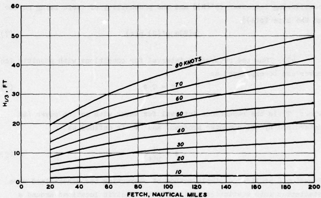
Figure 22. Growth of significant wave height as a function of wind speed and fetch (after SPM<sup>5</sup>)
