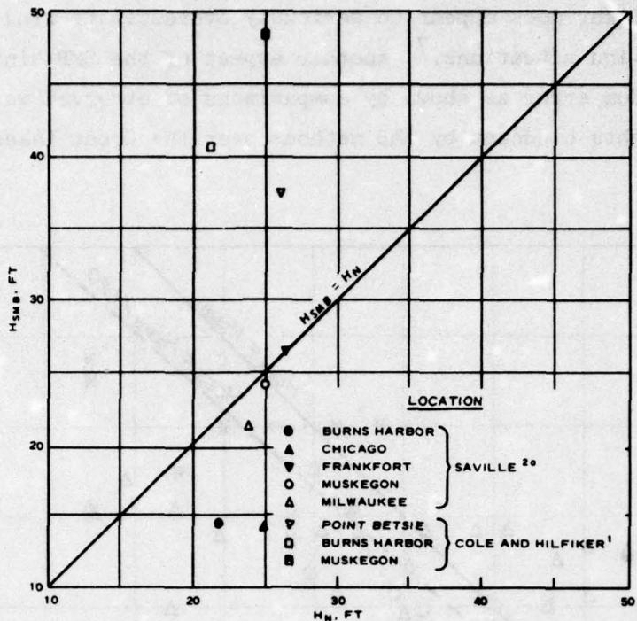
Figure 23. Wave heights for 20-yr return periods at sites on Lake Michigan as hindcast by Saville<sup>2a</sup> and Cole and Hilfiker<sup>1</sup> ( $H_{SMB}$ ) compared to wave heights for 20-yr return periods hindcast in the present study ( $H_N$ )
