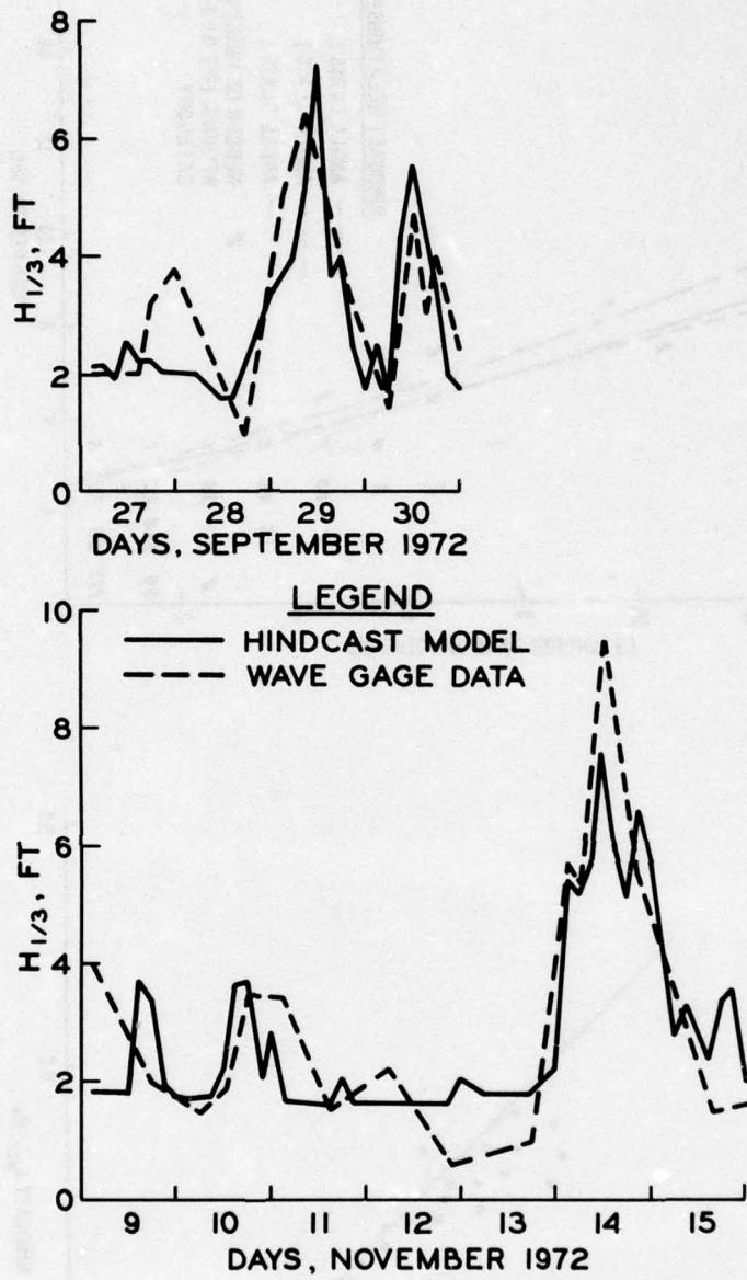
Figure B5. Comparisons of hindcast and observed sequences of significant wave height at Main Duck, with the best agreement shown at the top and the worst at the bottom
