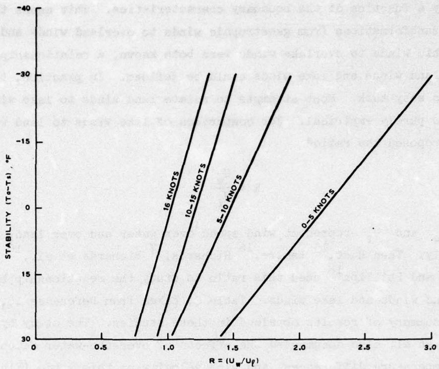
Figure 9. Characteristics of the ratio of overlake wind velocities to overland velocities for various wind speed classes as a function of air-water temperature (after Richards et al.<sup>10</sup>)
