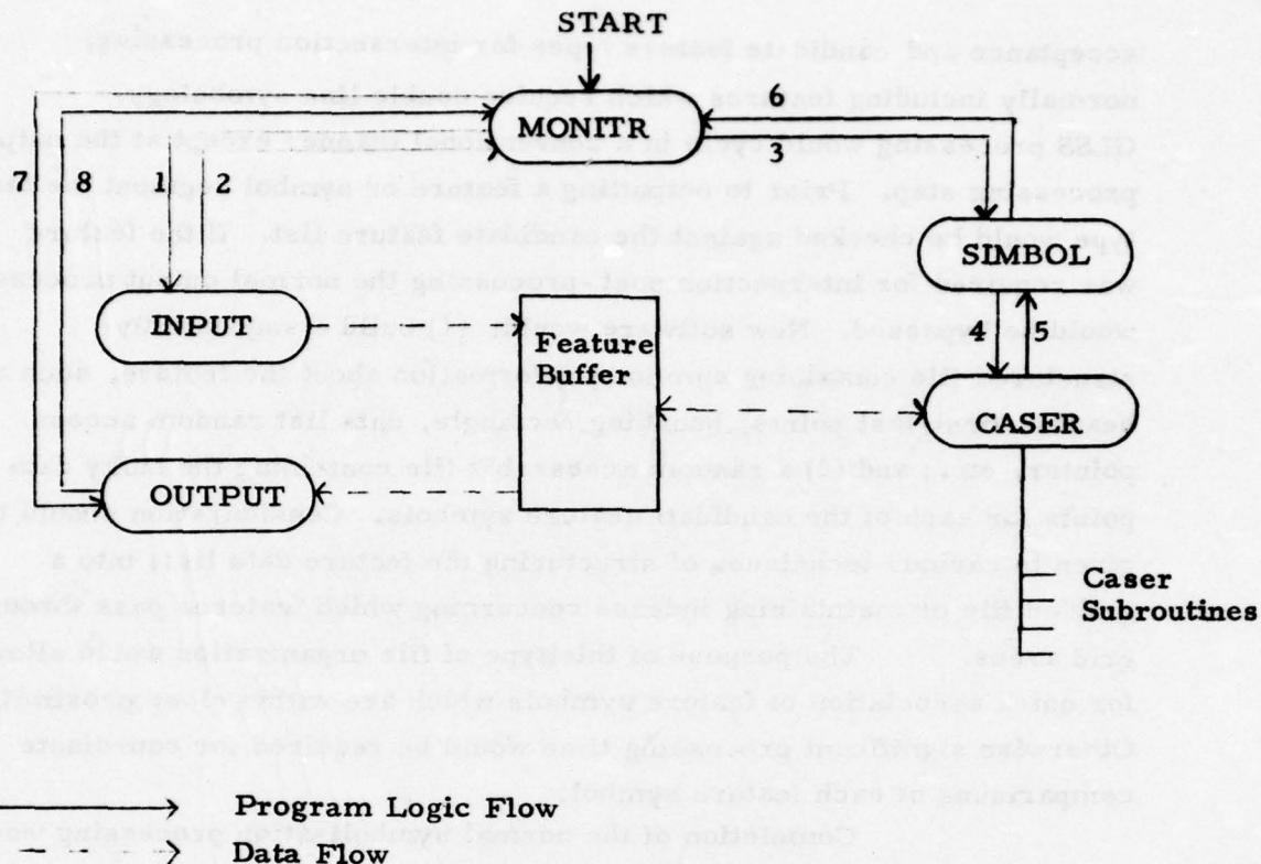
**Figure II-9 General Flow of Case Processing**
