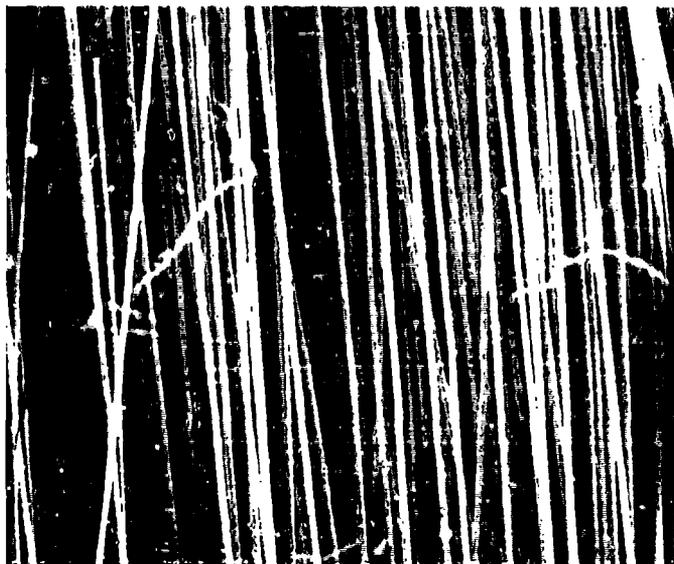
Figure 2. Surface layer of a typical glass-fiber/-epoxy composite after removal of resin.
