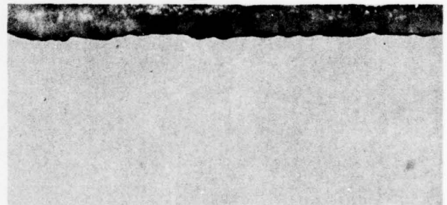
Ground with 9 μm Al 2 O 3 and 2.0-hour HF etch
