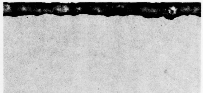
Ground with 9 μm Al 2 O 3 and 1.0-hour HF etch
