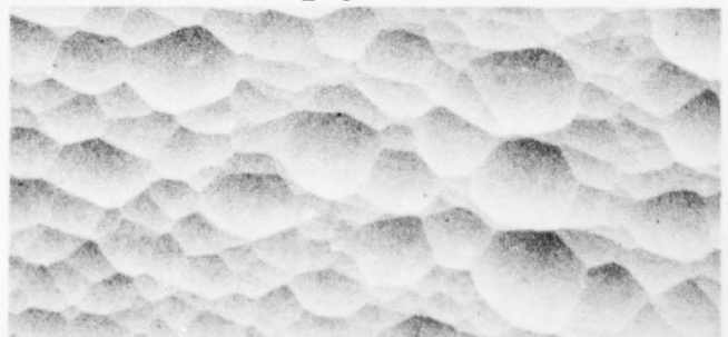
Ground with 9 \mu\text{m} \text{Al}_2\text{O}_3 and 2.5-hour HF etch
