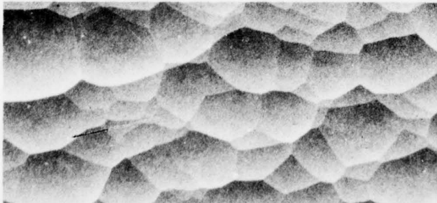
Corning 7940 fused-silica – scanning electron microscope micrographs. (300X magnification in all cases).
