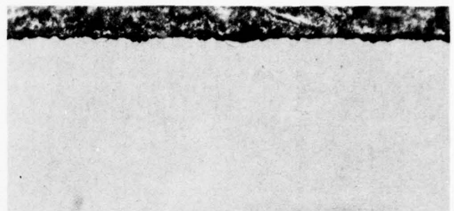
Ground with 9 μm Al 2 O 3 , no etching
