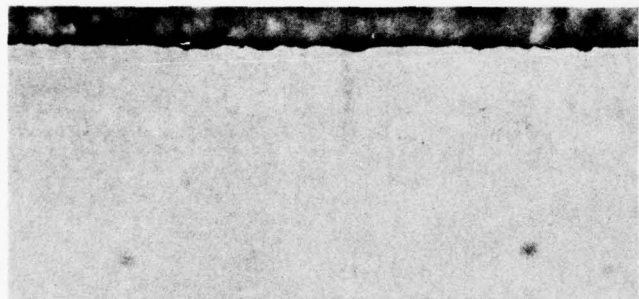
Ground with 3 μm Al 2 O 3 and 1.0-hour HF etch
