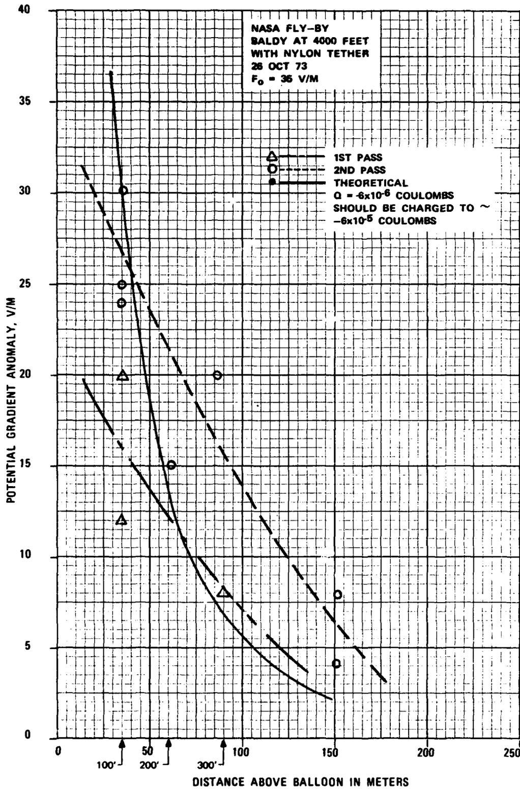
Figure 2.3 - Potential Gradient Anomaly Above Balloon, Nylon Tether - 26 Oct 73
