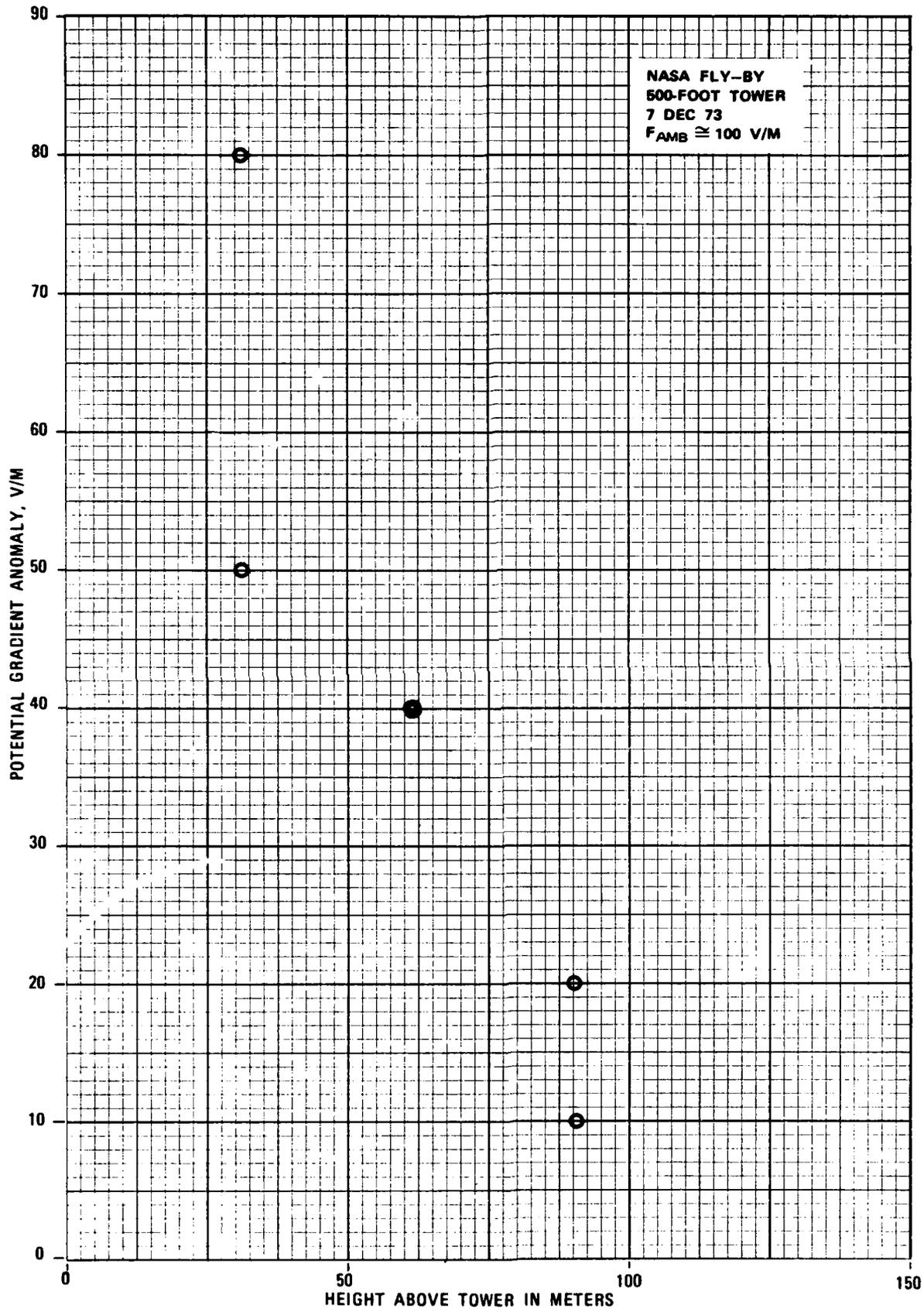
Figure 2.6 - Potential Gradient Anomaly Above 500-Foot Tower
