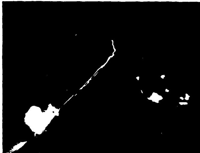
Figure 6. Typical high voltage-high current multiple discharge. The high voltage was applied at the top with the high current added at the bottom.
