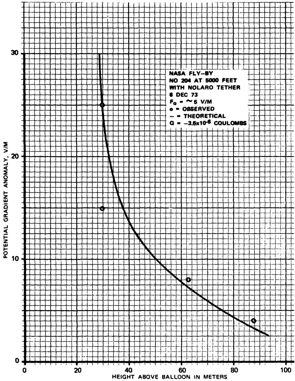
Figure 2.5 - Potential Gradient Anomaly Above Balloon, Nolaro Tether - 6 Dec 73
