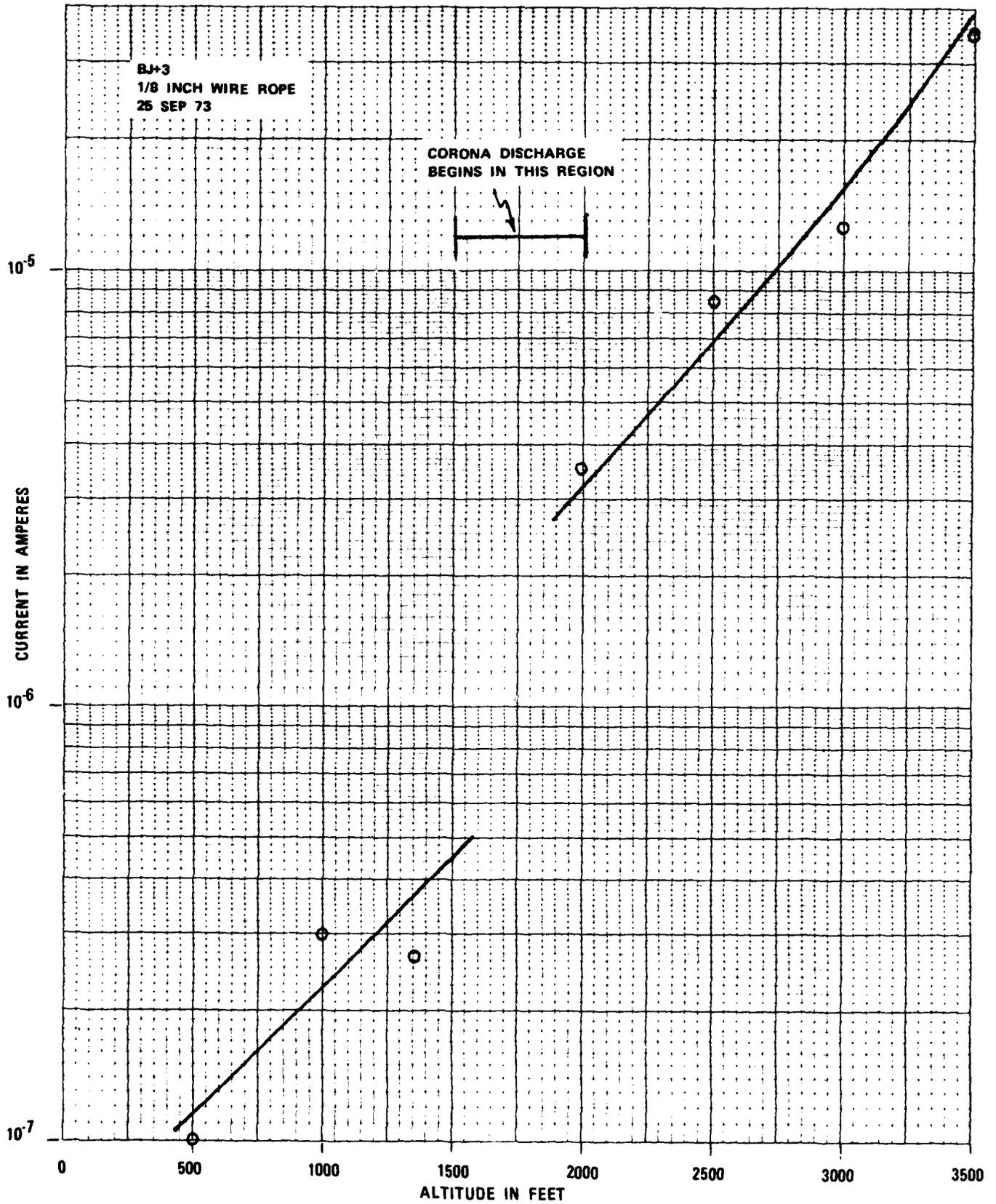
Figure 3.1 - Tether Current vs Balloon Altitude, BJ+3 - 25 Sep 73
