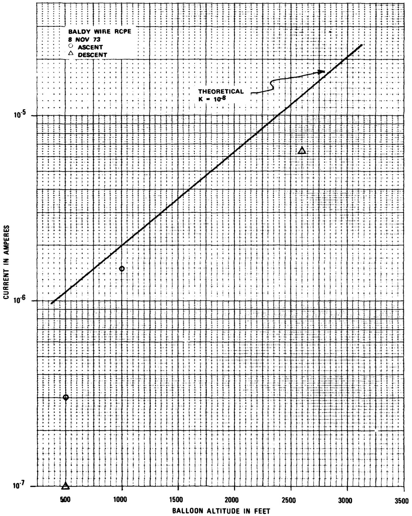
Figure 3.5 -- Tether Current vs Balloon Altitude, Baldy - 8 Nov 73
