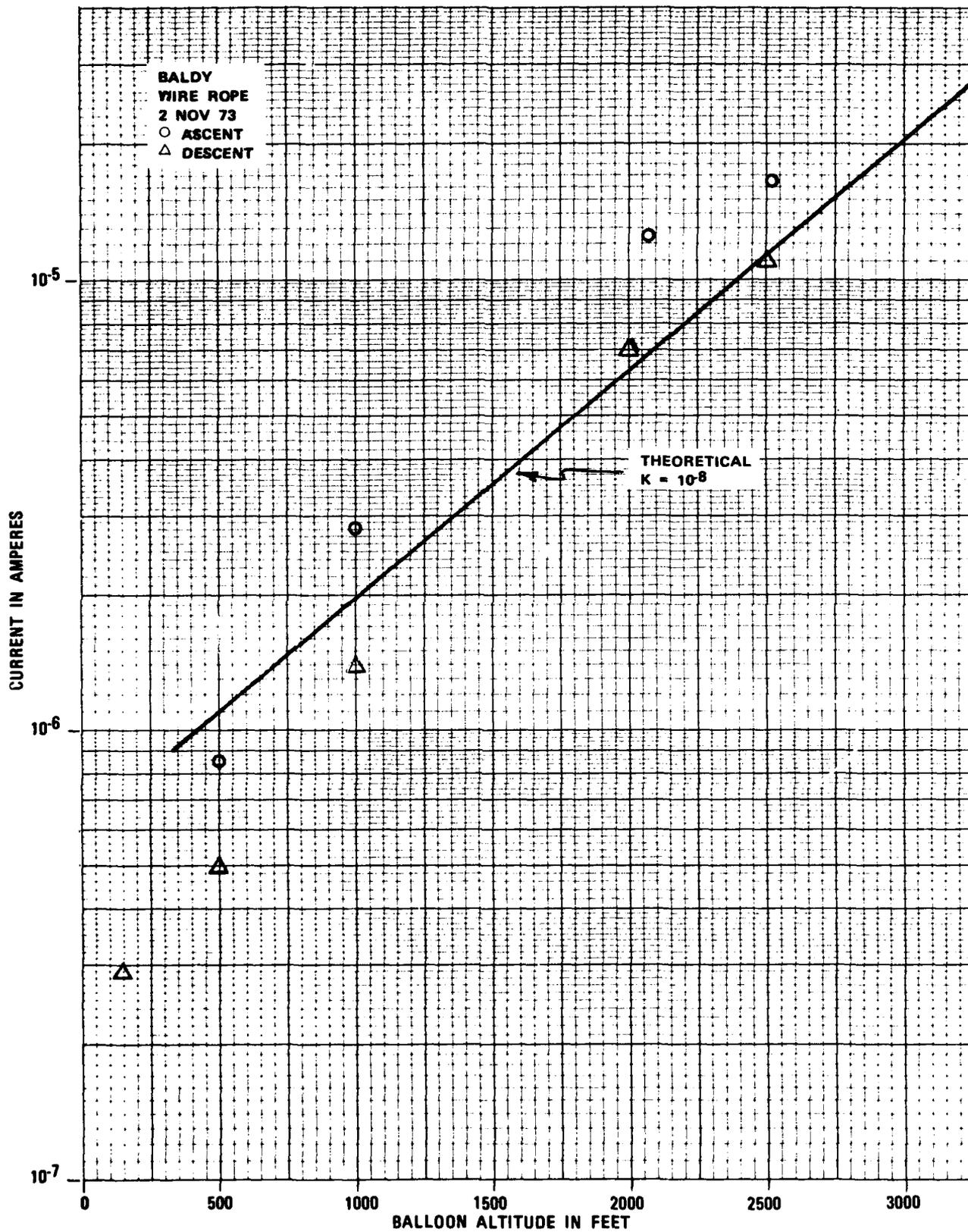
Figure 3.4 - Tether Current vs Balloon Altitude, Baldy - 2 Nov 73
