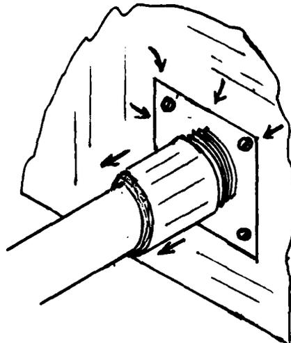
Figure 4. The lightning current should be forced to flow externally through a peripherally bonded connector.
