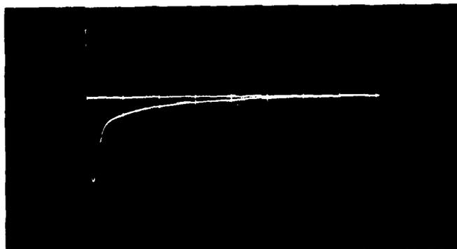
Figure 8(c). Longer waveform applied from a 281 uf. bank. Calibration 7 Ka. and 100  $\mu$ sec. / large division.
