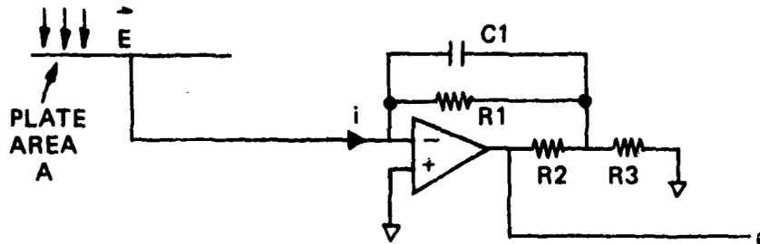
Originally, the purpose of  $C_1$  was to act as a low-pass filter for the air-earth current measurement. It became apparent, on examination of the data that the circuit was also acting as a charge amplifier, hence as a "slow antenna" with the response time limited essentially by the slow rate of the amplifier. For the circuit actually used in practice, the following relationship was obtained:
