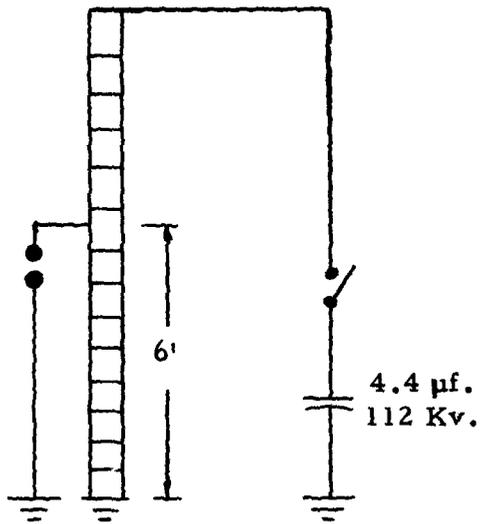
Voltage across unprotected ladder measured by spark gap shown on ladder at left.
