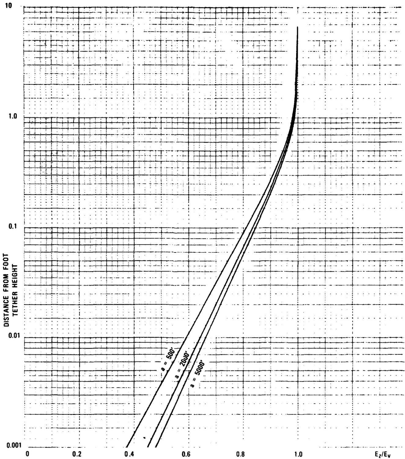
Figure A.1 - Suppression of Vertical Field ( $E_z$ ) on the Ground at Some Distance ( $R$ ) from the Tether Point With a Balloon at Altitude ( $a$ )
