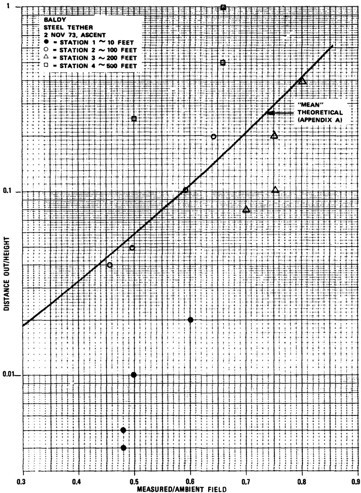
Figure 4.1 - Data Plot of Distance/Height vs Measured/Ambient Field, Ascent
