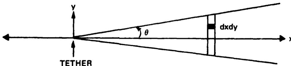
Let the "unspread" line charge density be  $\lambda$ ; it is given by  $\lambda = i/\bar{u}$  where  $i$  is the corona current and  $\bar{u}$  is the mean wind velocity. Assume further a "top hat" distribution for the charge rather than a Gaussian.
