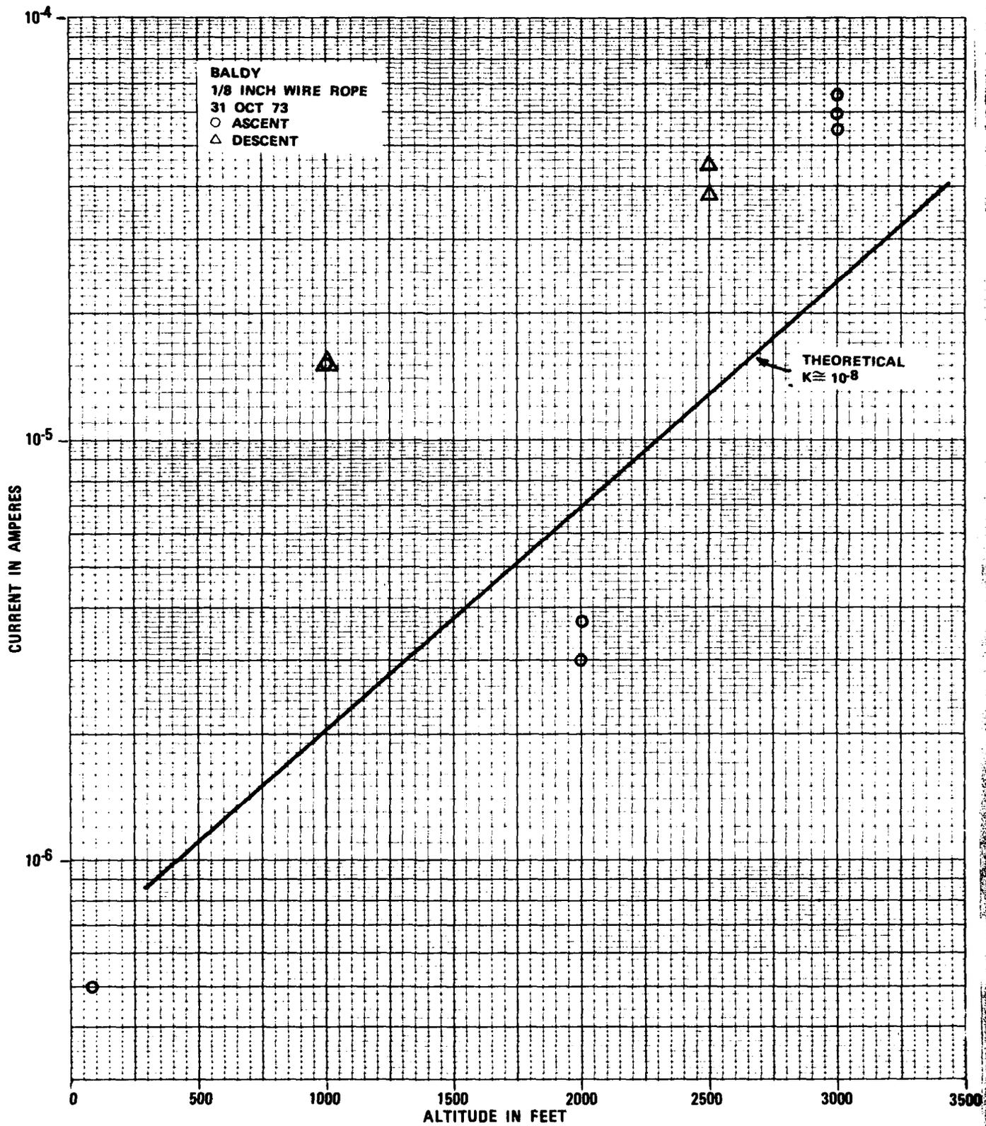
Figure 3.3 - Tether Current vs Balloon Altitude, Baldy - 31 Oct 73
