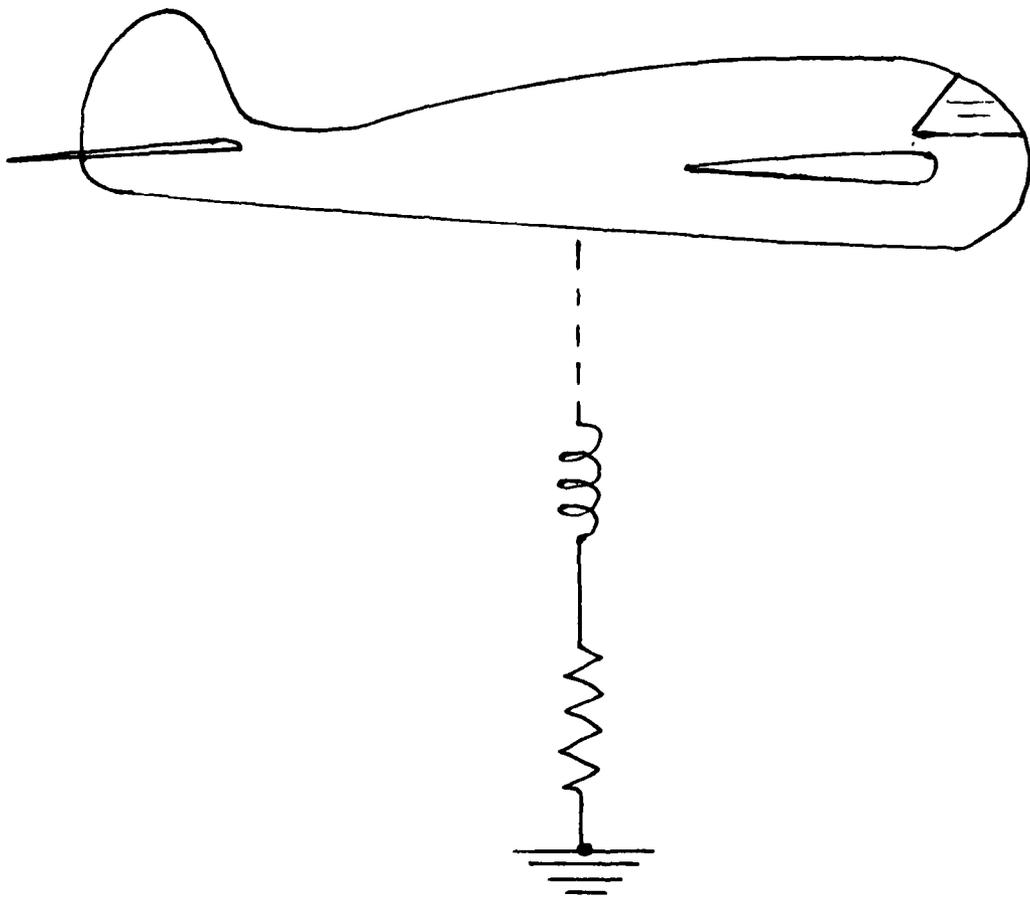
Figure 2. The external potential of a good conducting metal enclosure, such as an aircraft, has little effect on the relative potentials inside. Grounding has little effect and is not necessary to protect those inside the enclosure.
