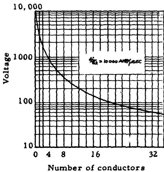
Voltage as function of number of shield wires.
