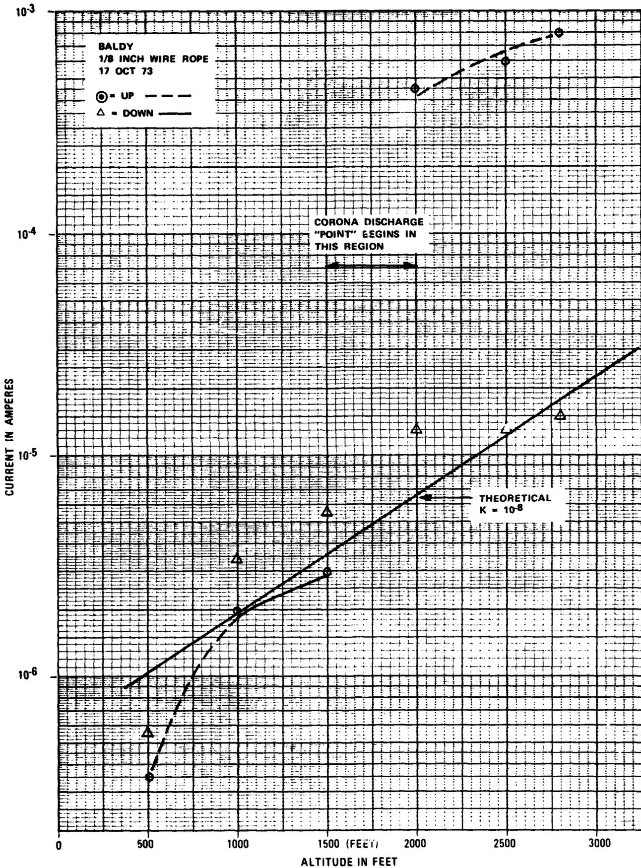
Figure 3.2 - Tether Current vs Balloon Altitude, Baldy - 17 Oct 73
