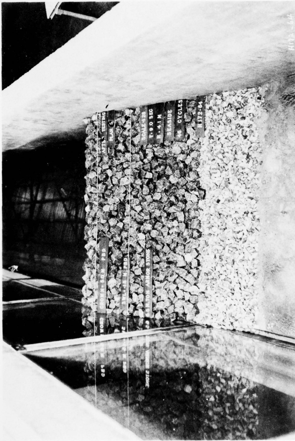
Photo 30. Seaside view of Plan 5 in the deeper water location after attack of 9-sec, 4.1-m waves at a swl of +1.50-m PBD
