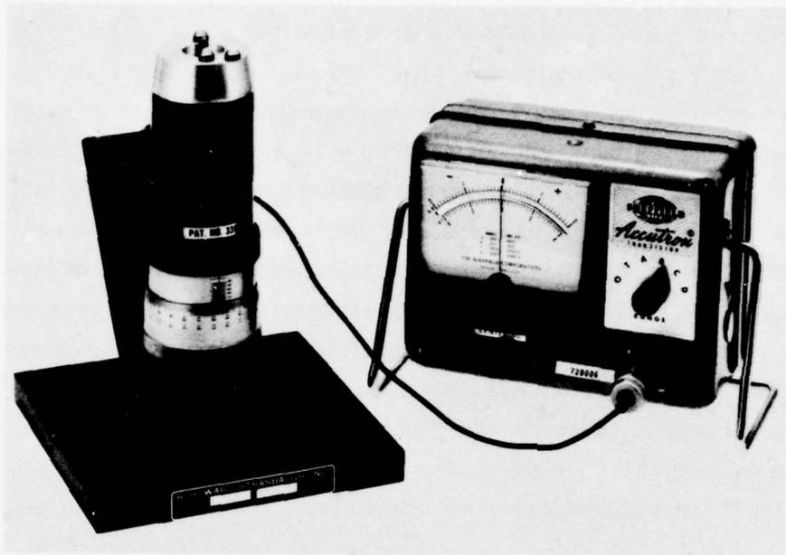
Figure 10. Electronic Sagittal Micrometer
