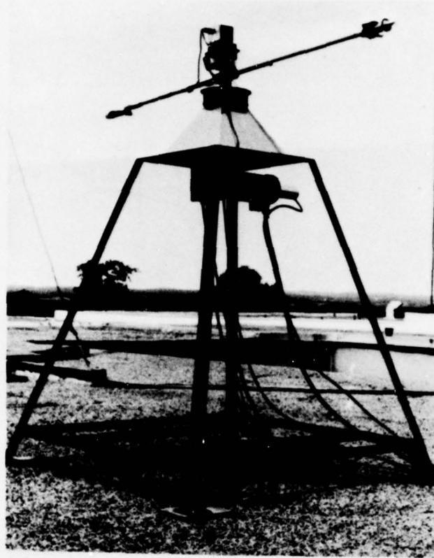
FIG. 14: WHIRLING ARM APPARATUS MOUNTED ON LABORATORY ROOF
