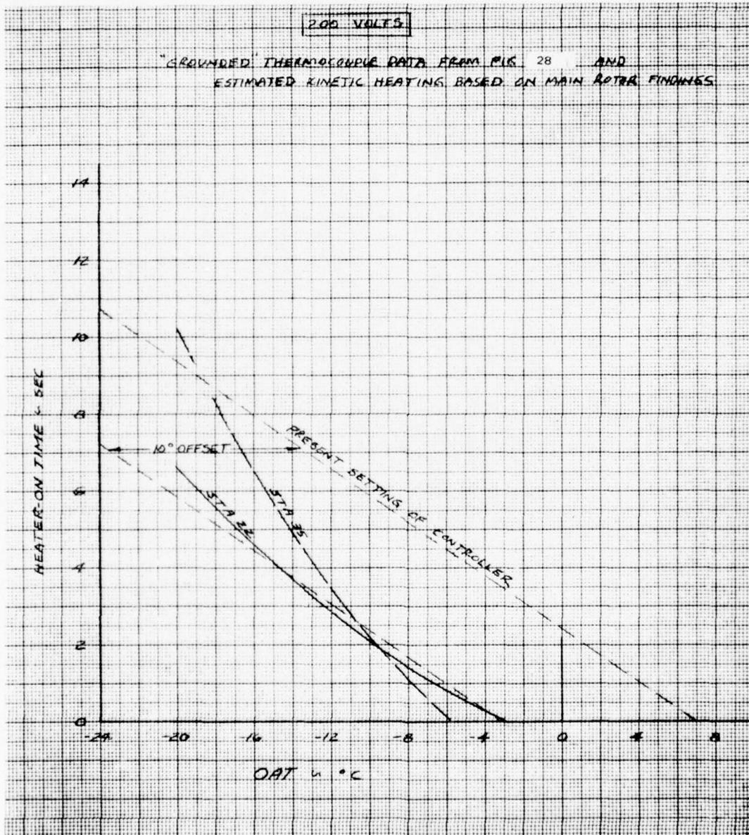
Figure 29. Tail Rotor Heater-On Time to Raise Surface Temperature to 0°C
