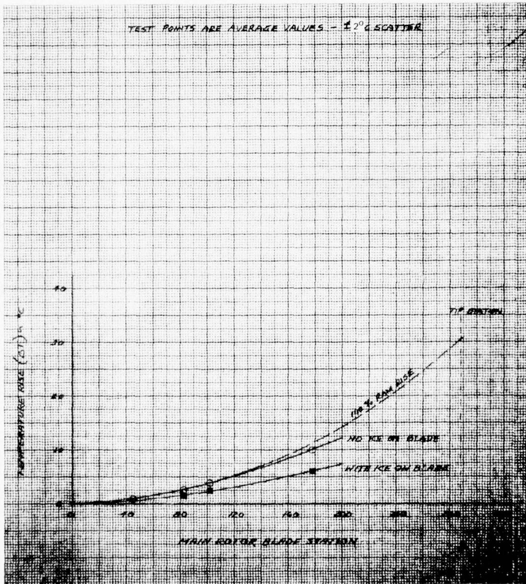
Figure 26. Temperature Rise Due to Kinetic Heating
