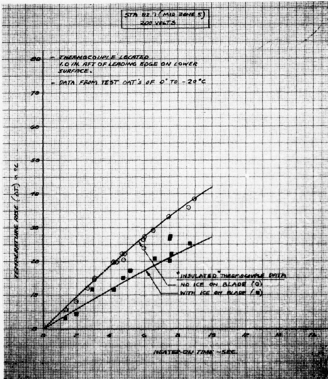
Figure 22. Main Rotor Blade Surface Temperature Rise vs Heater-On Time - Sta. 82.7
