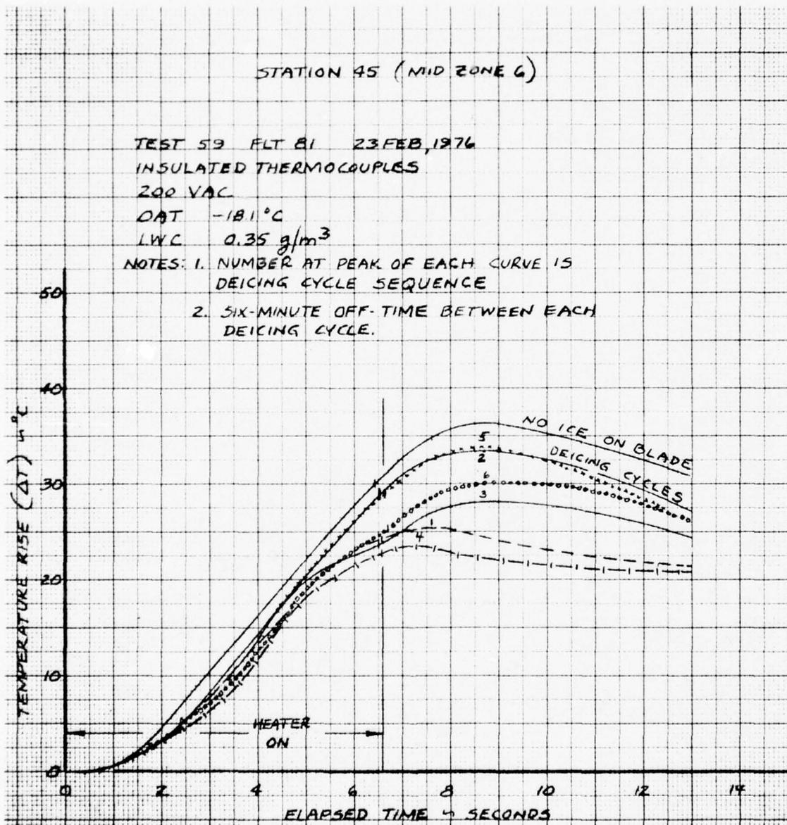
Figure 25. Time History of Blade Temperature Rise During Several Deicing Cycles in the Same 30-Minute Spray Cloud Run
