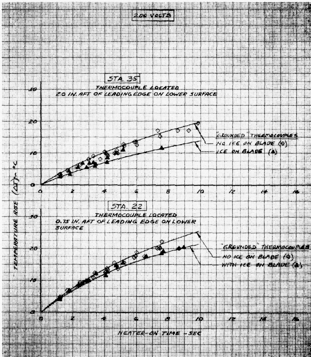
Figure 28. Tail Rotor Blade Surface Temperature Rise vs Heater-On Time
