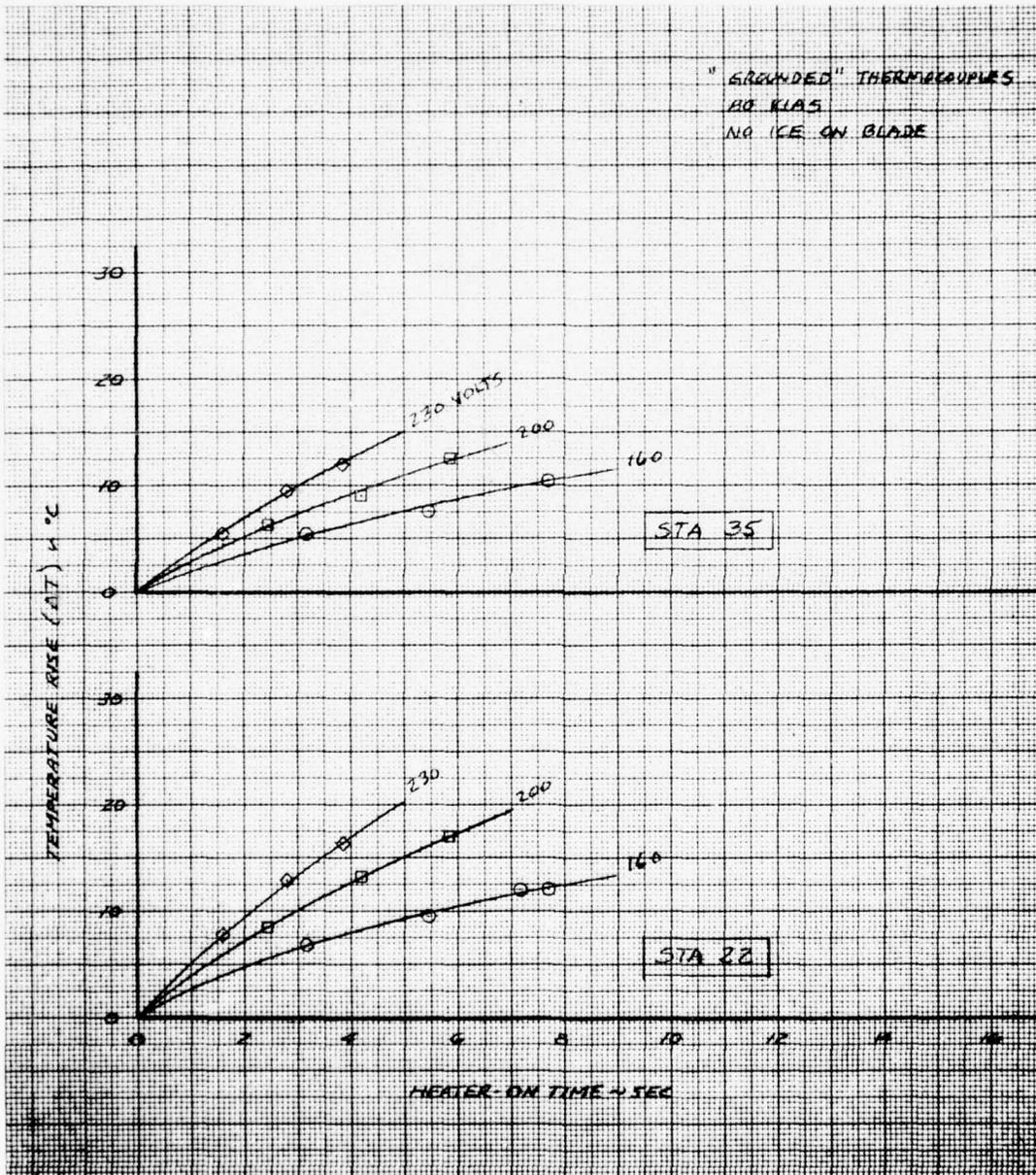
Figure 31. Tail Rotor Blade Surface Temperature Rise for Different Voltages
