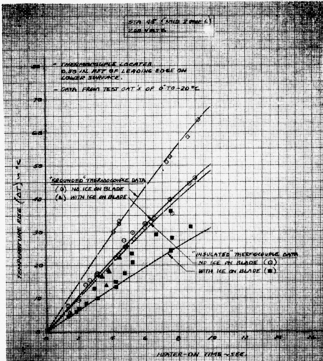
Figure 21. Main Rotor Blade Surface Temperature Rise vs Heater-On Time - Sta. 45
