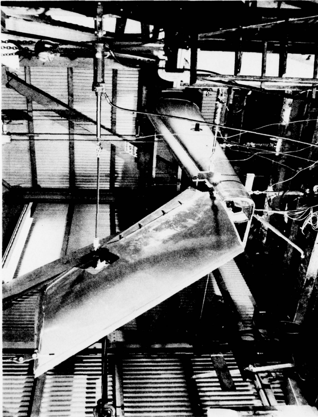
Figure D-1. View of Test Setup of AH-1G Flight Test Tail Boom Static Proof Test.
