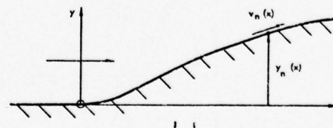
FIG.2.2A LOWER-WALL/STREAMLINE CONTOUR, AND COMPARISON BETWEEN THE EXACT WALL PRESSURE DISTRIBUTION AND THE WALL DISTRIBUTION C_{pi} COMPUTED WITH THE SOURCE/SINK GENERATION OF IMAGINARY FLOWFIELD.
