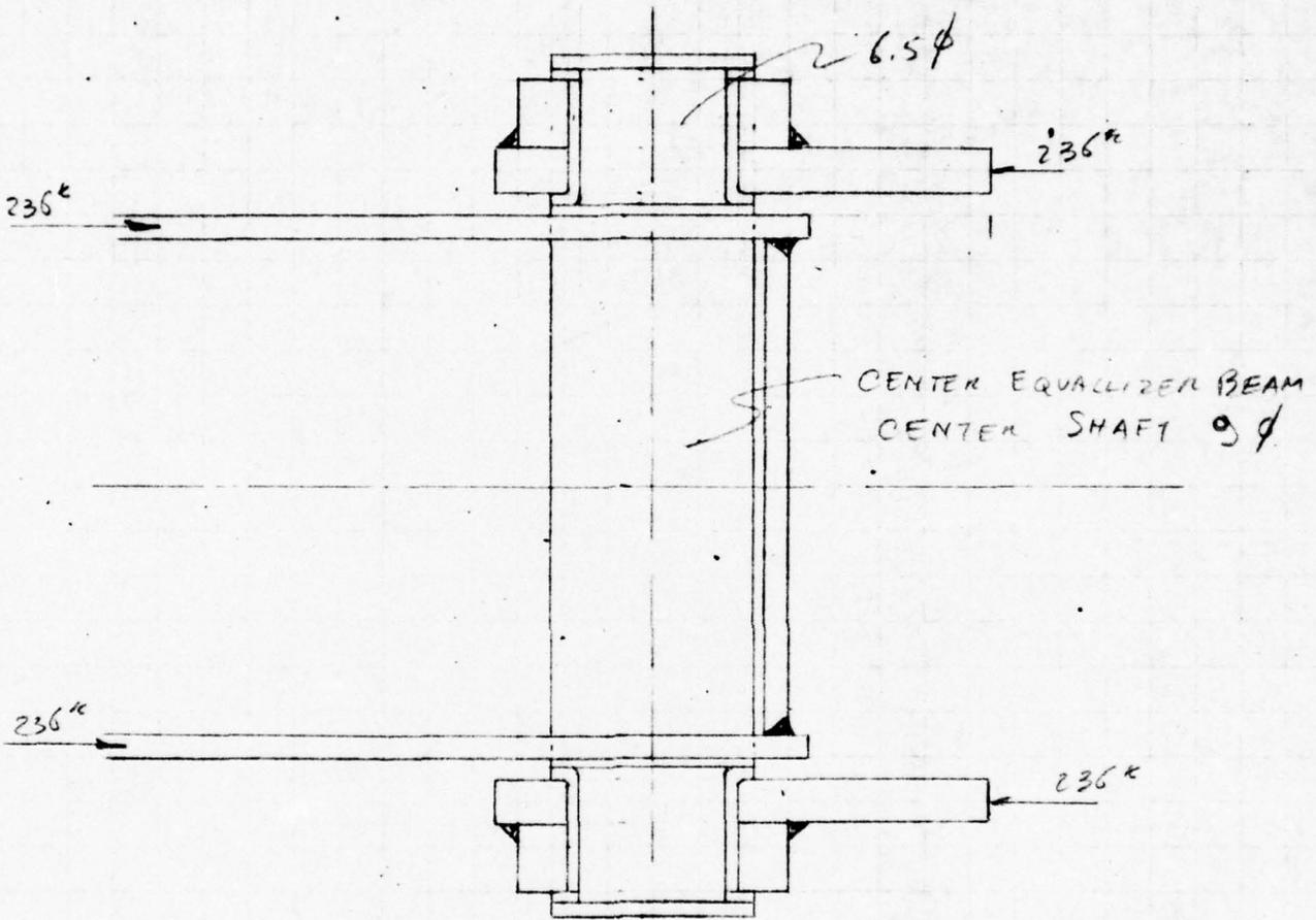
BEARING IN GIRDER  $\frac{236}{1 \times 2} = 9.8 \text{ KSI OK}$
