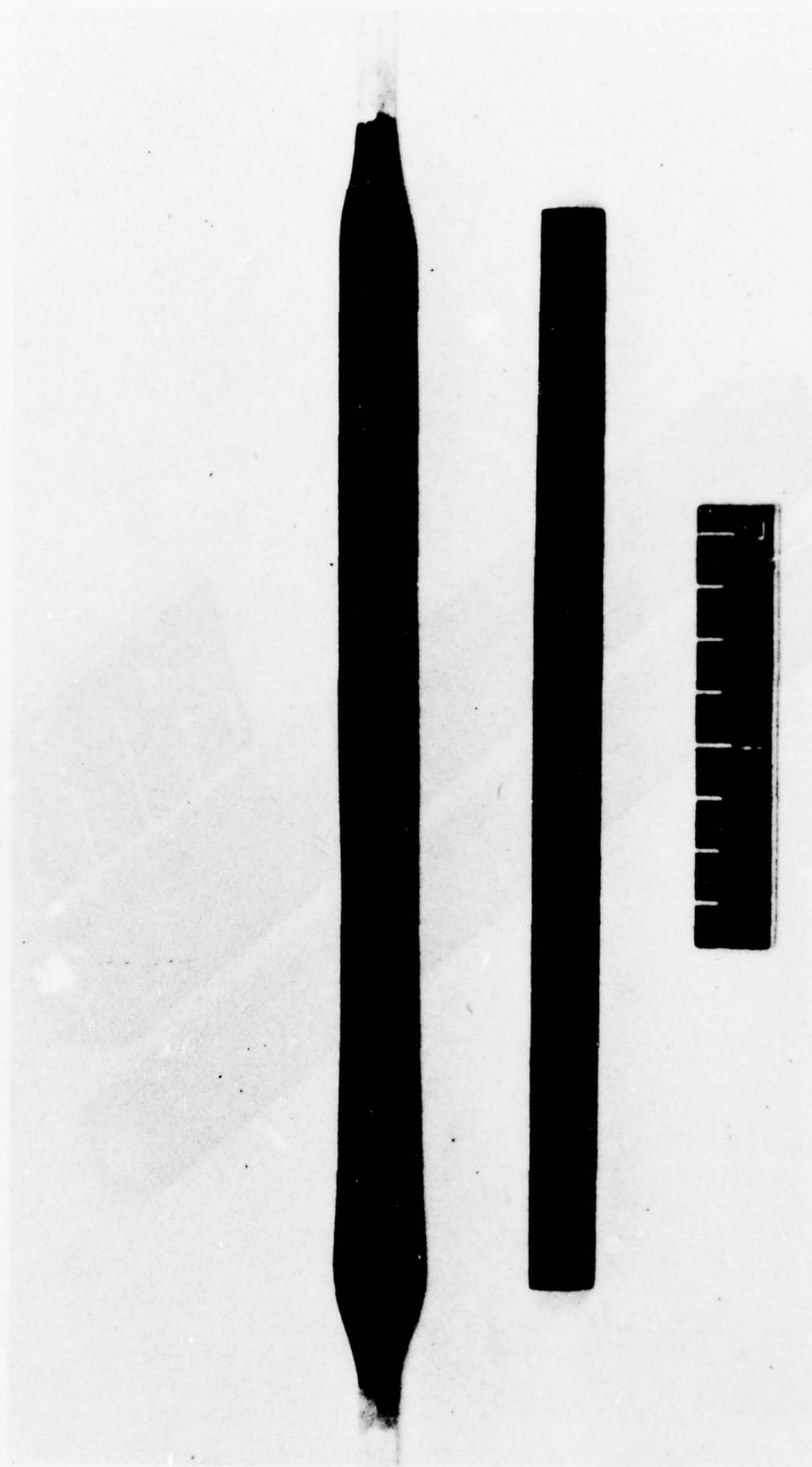
Figure 9. Arc Plasma Ferrite Phase Shifter, as Deposited and after Machining
