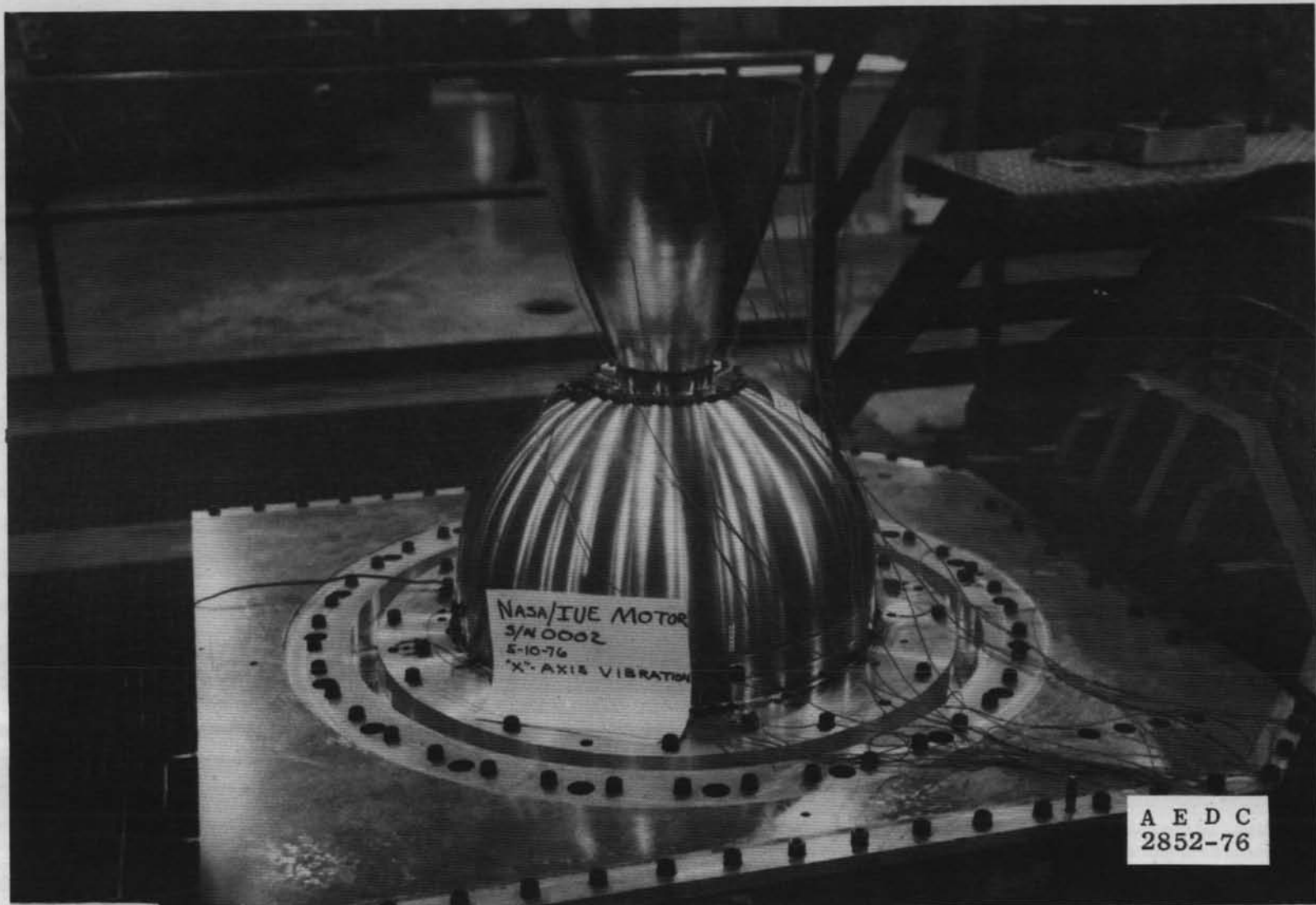
Figure 11. X-axis motor installation photographs.
