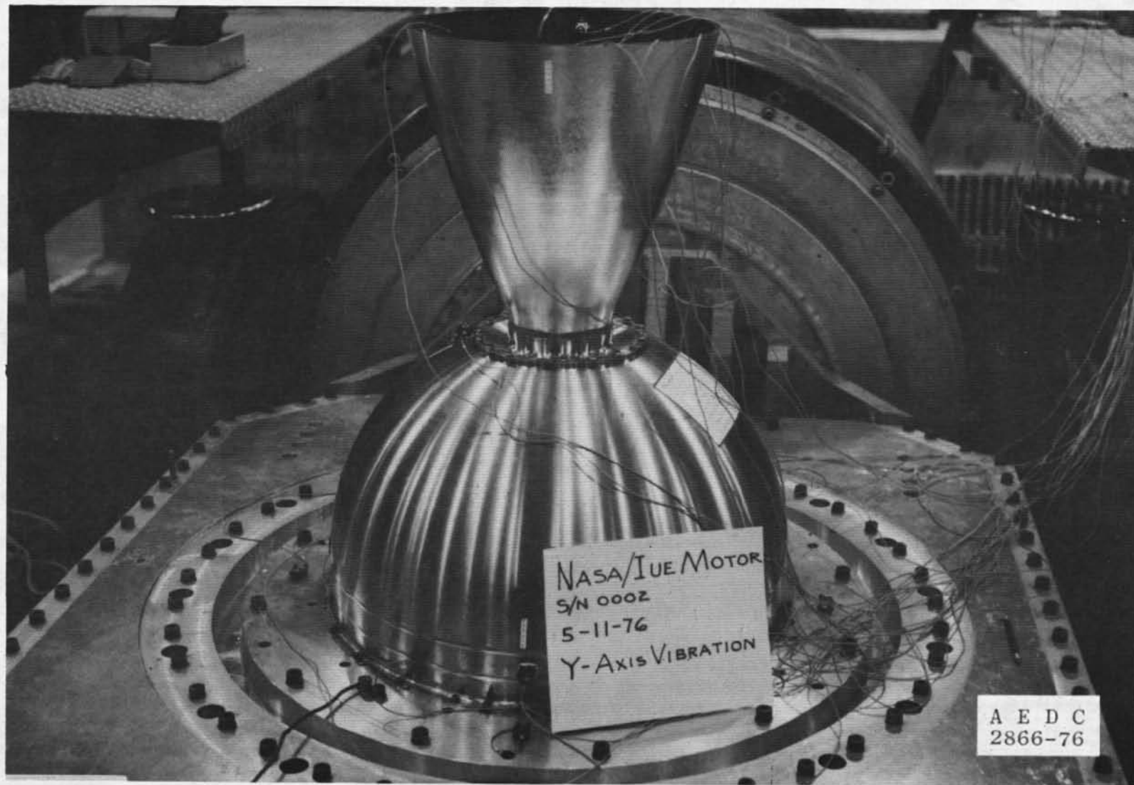
Figure 16. Y-axis motor installation photographs.
