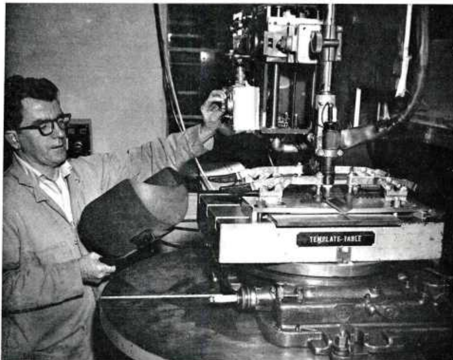
Figure 1. GTA welding setup for parallel and intersecting welds
