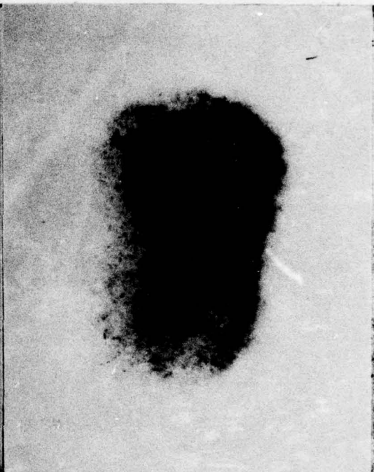
Fig. 18. Far-field intensity patterns of F_1 - F_3 resonator with NaCl flat in cavity.
